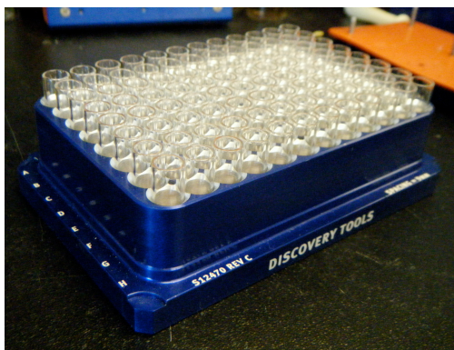
Figure 3.33. Screening plate containing 96 vials.
