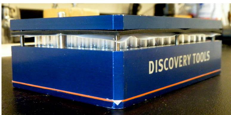
Figure 3.37. Plate used for GC-MS analysis.
