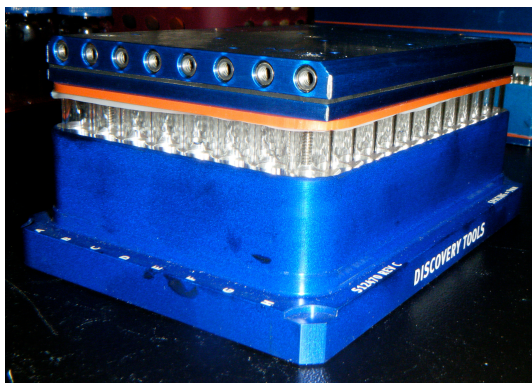
Figure 3.34. Assembled screening plate with top plate.
