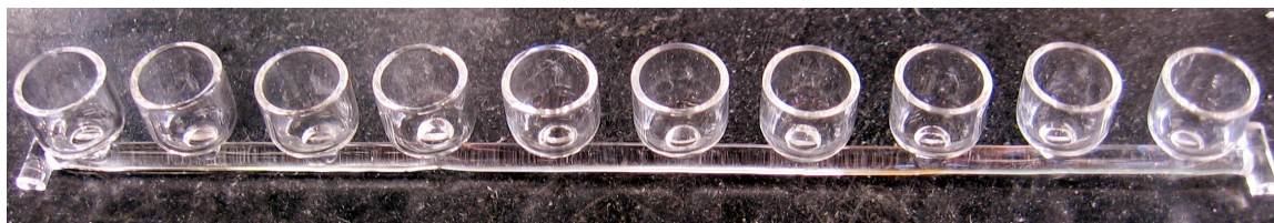
Figure 2.4. Initial screening apparatus. Each sample holder has a volume of approximately 1 ml.
