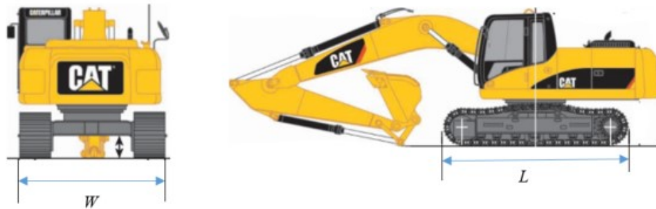
Figure 5.5. Defining body factor for the excavator.
