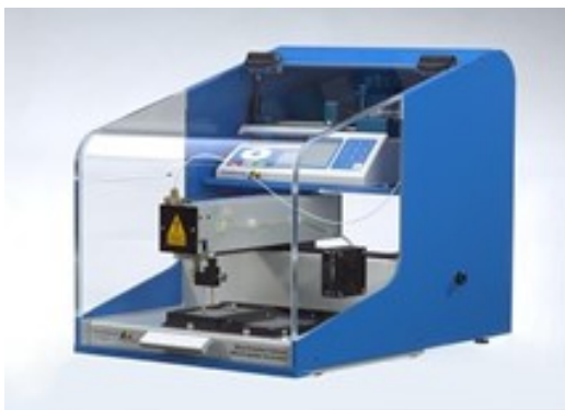
Figure 5.1. SunChrom SunCollect™ by Separation Associates for MALDI tissue imaging.
