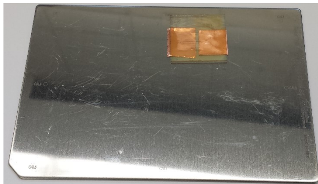
Figure 5.3. Picture of Si GLAD film with tissue samples attached to MALDI plate with double sided sticky copper tape.
