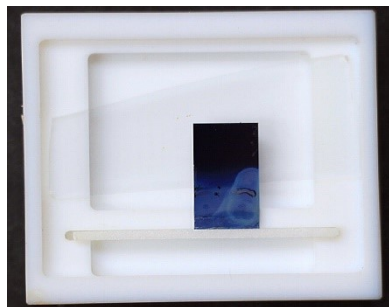
Figure 4.1. Horizontal UTLC development chamber with silica GLAD film.
