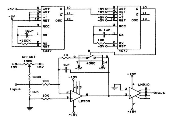
Appendix A-4. Schematic circuit of the full-wave precision rectifier.
