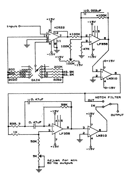
Appendix A-3. Schematic circuit of the main instrumentation amplifier.
