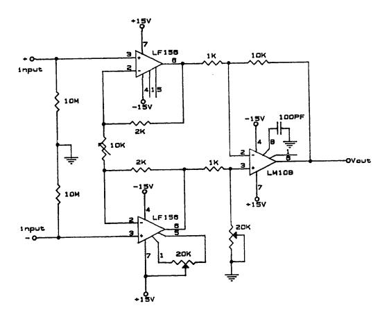
Appendix A-2. Schematic circuit of the high-input impedance differential amplifier (pre-amplifier).
