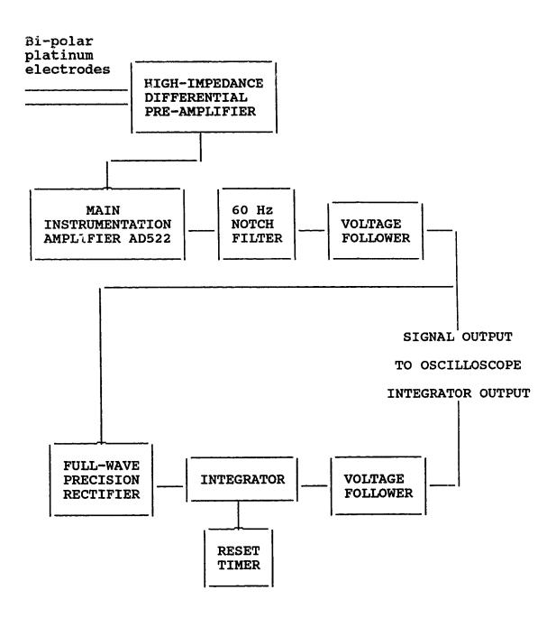
Appendix A-1. Block diagram of a bio-electric amplifier system. The system was used for recording the nerve activity.
