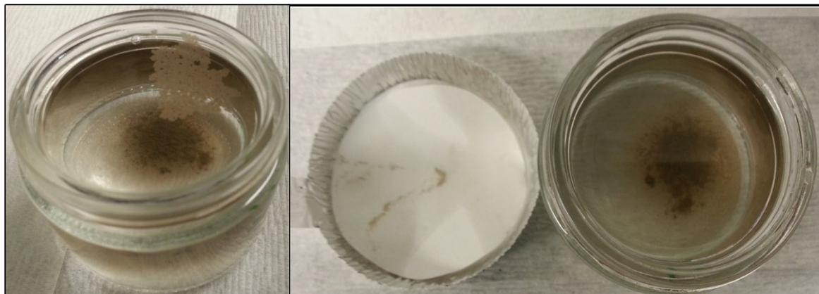
**Figure 10: Film Flotation Apparatus**
