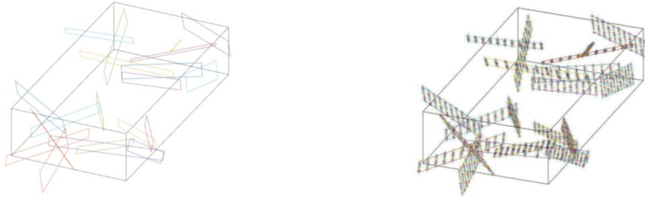
Fig. 3.5. Segmentation scheme for 3D fracture planes.
