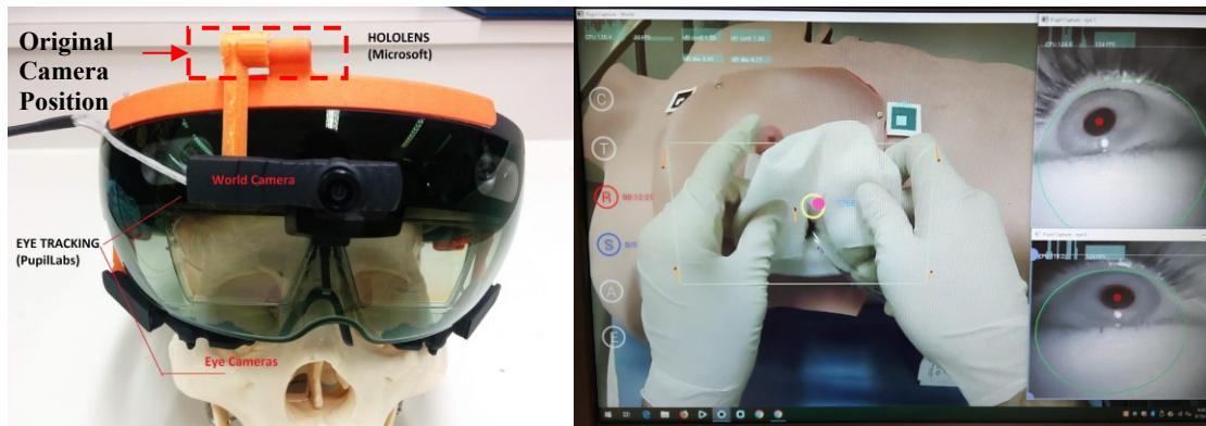
Figure 4.4. Left: AR headset with the new position of the world camera of the add-on eye tracker. Right: Screenshot of the visualization of eye gaze, now more accurate.
