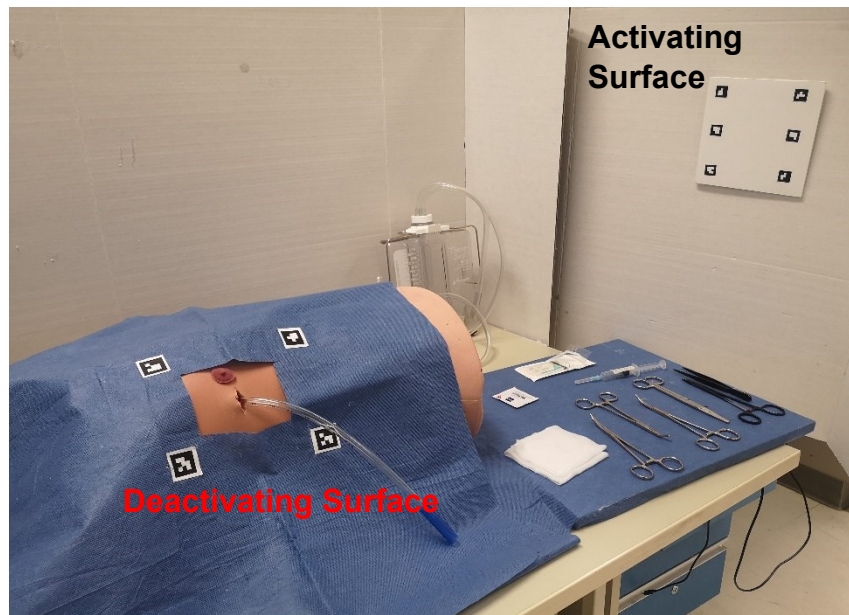
Figure 6.1. Workstation, including the chest tube model, instruments, and the surfaces placed to activate and deactivate the display of information on the AR goggles using gaze positions within the surfaces
