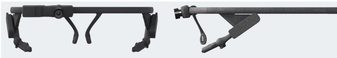
Figure 4.2. Pupil Lab head-mounted eye tracker with an accuracy of 0.60^\circ and a precision of 0.02. It is retrieved from https://pupil-labs.com/products/core/tech-specs .
