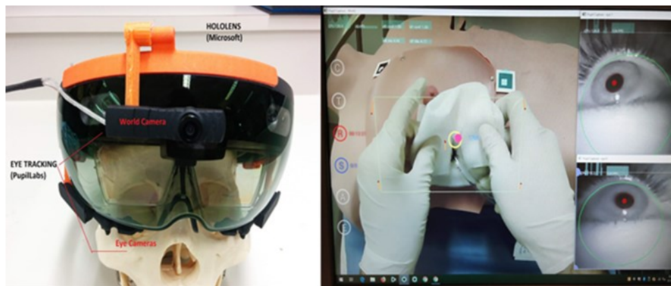
Figure 5.1. Left: AR headset with a set of eye tracker. Right: Screenshot of the visualization of eye gaze during the procedure
