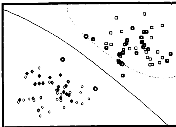
Figure 5-6: Decision boundaries for the SVM on data (a). Testing points are the bold patterns. Support vectors are indicated with a circle around the corresponding patterns.
