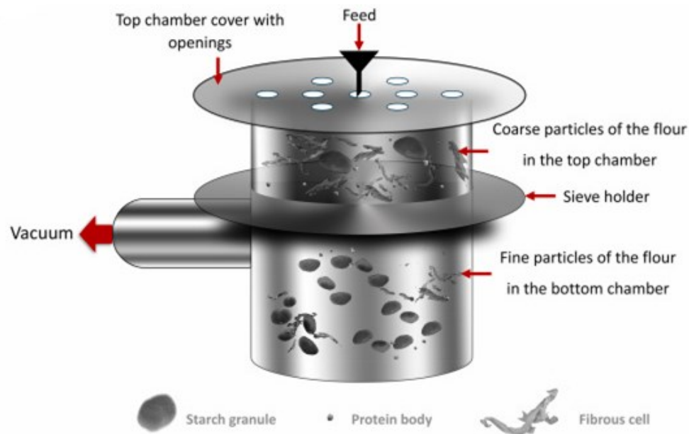
Figure 2-4 Simplified overview of air-currents assisted particle separation (ACAPS) of starch macro components. Republished with permission of ELSEVIER from [Journal of Food Engineering, Potential of air-currents assisted particle separation (ACAPS) technology for hybrid fractionation of clean-label faba bean ( Vicia faba L.), Jeganathan et al., 2023]; permission conveyed through copyright Clearance Center, Inc.
