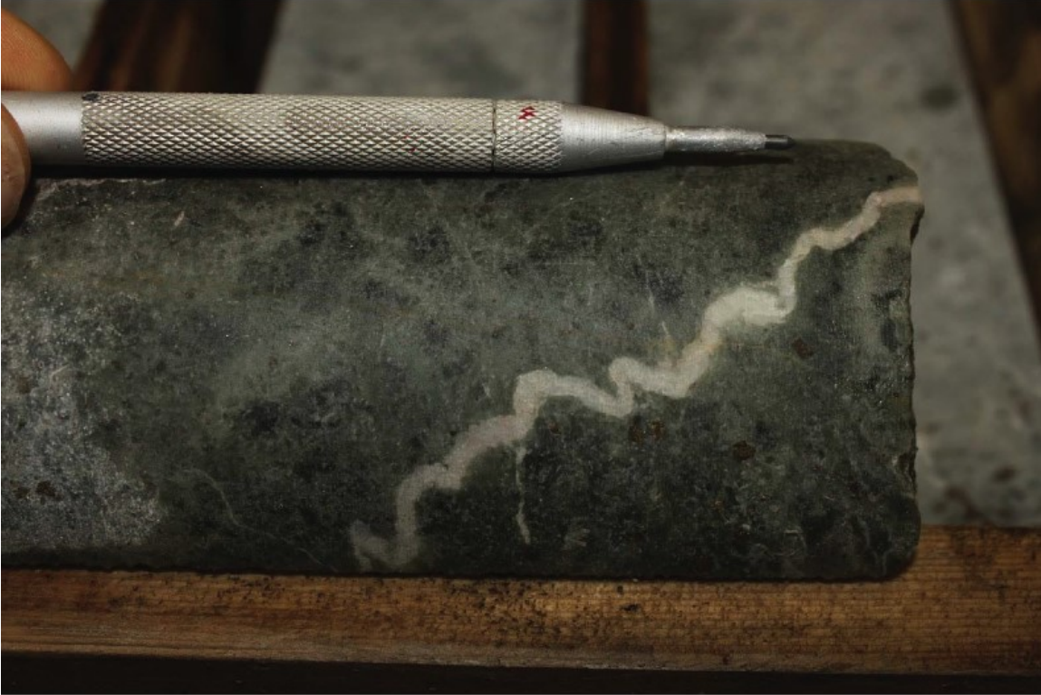
Figure 15: Ptygmatic vein within lapilli tuff (SU-158 at 47m: 426483E, 6257441N, 1498m)
