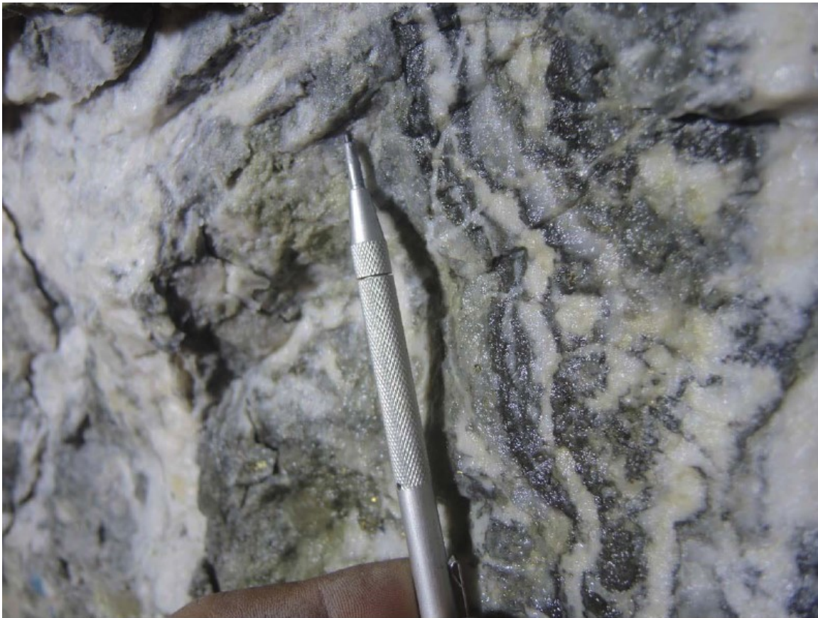
Figure 14: Crustiform banding within silica-flooded quartz stockwork-breccia vein (underground: 426647E, 6258039N, 1345 m)
