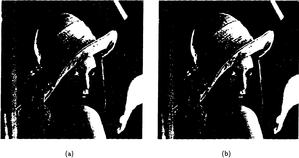
Figure 5.7: Reconstructed Lena image at 0.214 bpp from (a) SPIHT and (b) WP/HVS Pyramid.
