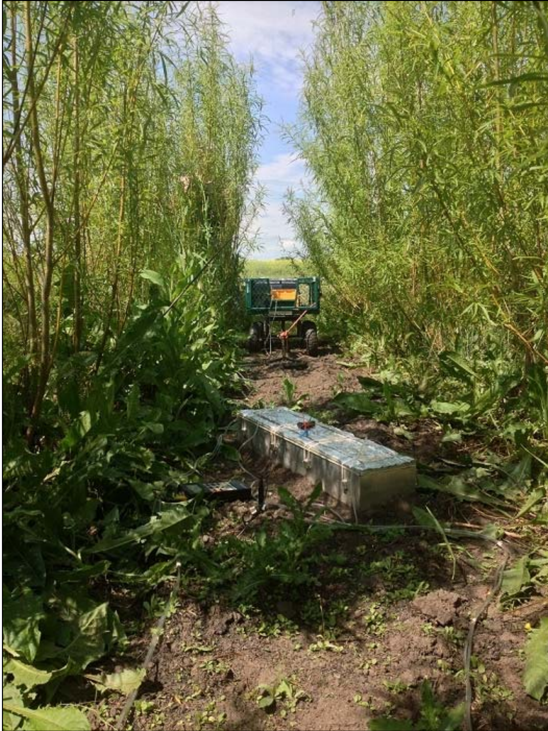
Figure 3-3: The non-steady closed chamber system comprised of both photoacoustic monitor and static chamber in connection.
