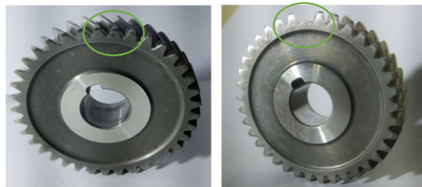
Fig. 3.22: The gear before and after the run-to-failure experiment. [76], [134]
