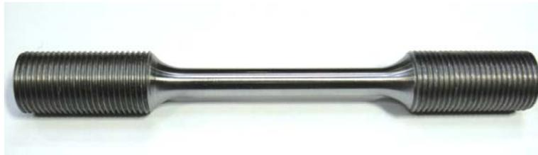
**Figure 3.5 Cylindrical-threaded elevated temperature test specimen**
