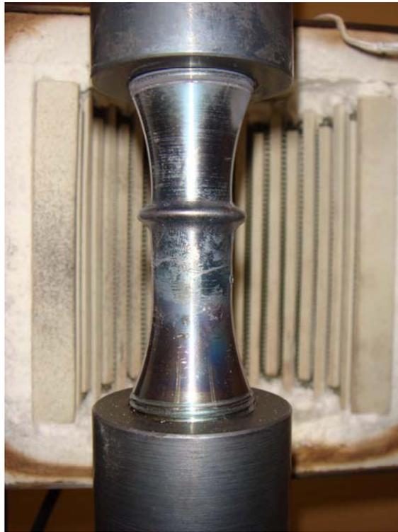
**Figure 4.21** Picture of collapsed tubular specimen
