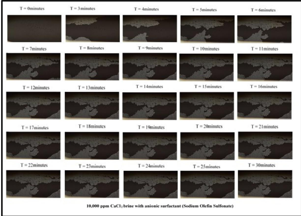
**Figure 4-21: Flooding results in 10,000 ppm CaCl<sub>2</sub> brine and anionic surfactant with the homogeneous micromodel**
