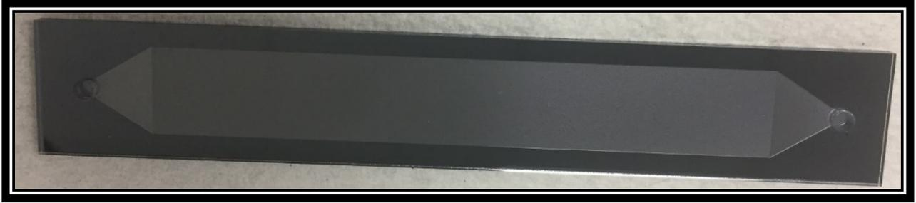
**Figure 3-9: Fabricated homogeneous micromodel**
