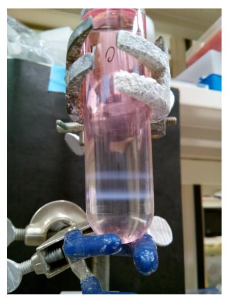
Figure 4- 1. Viral bands generated by Vertrel<sup>®</sup> XF-CsCl density-gradient centrifugation.
