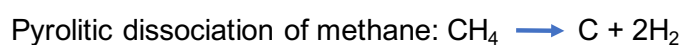
Figure 3.7 Chemical process of graphite formation from pyrolytic methane dissociation. Based on (Kwiecinska, B., and Petersen, H.I., 2004, p. 106)
