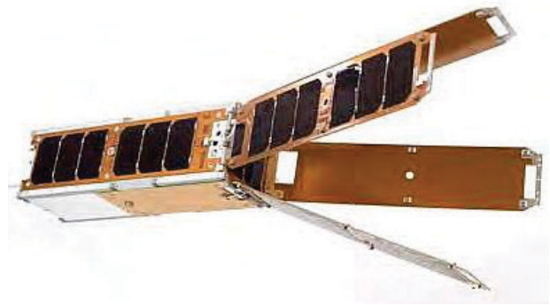
b) Space Dart Configuration (Reprinted [13], [59], photo credit Pumpkin Inc.)
