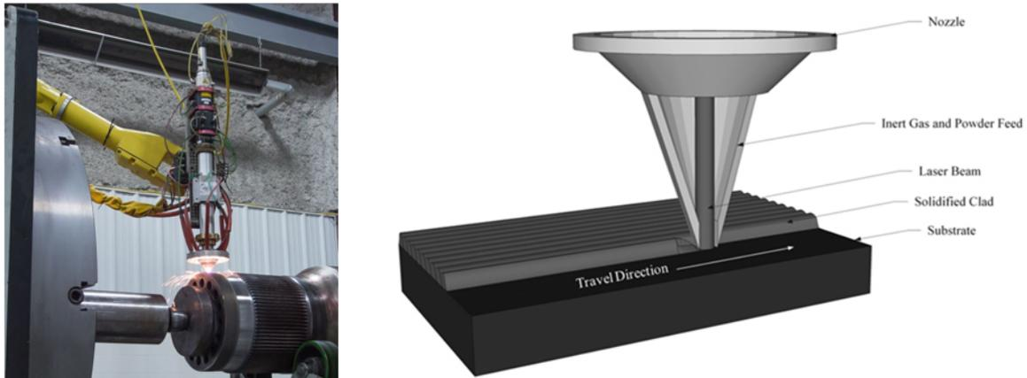
**Figure 1.1:** Left: Large mining component being manipulated with a CNC system relative to a robotic laser assembly. Right: Schematic of a typical coaxial laser system.
