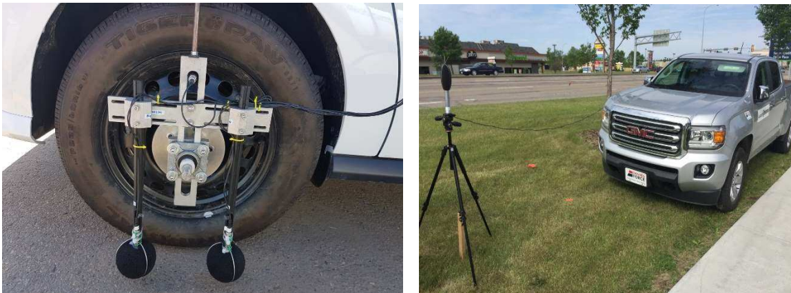
Figure 17a, 17b OBSI Measurement Set Up and Road Side Sensors along Corridor
