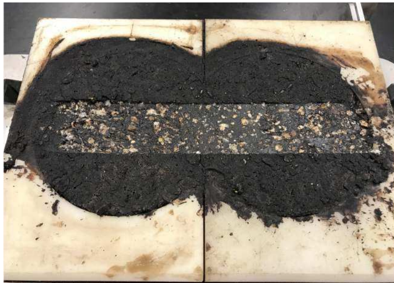
Figure 28 - SMA/Microsurfacing Sample After Hamburg Wheel [40]
