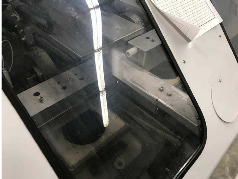
Figure 21 - University of Alberta Hamburg Wheel Tracker [40]
