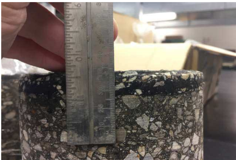
Figure 25 - Microsurfacing Core (16 mm of Microsurfacing)
