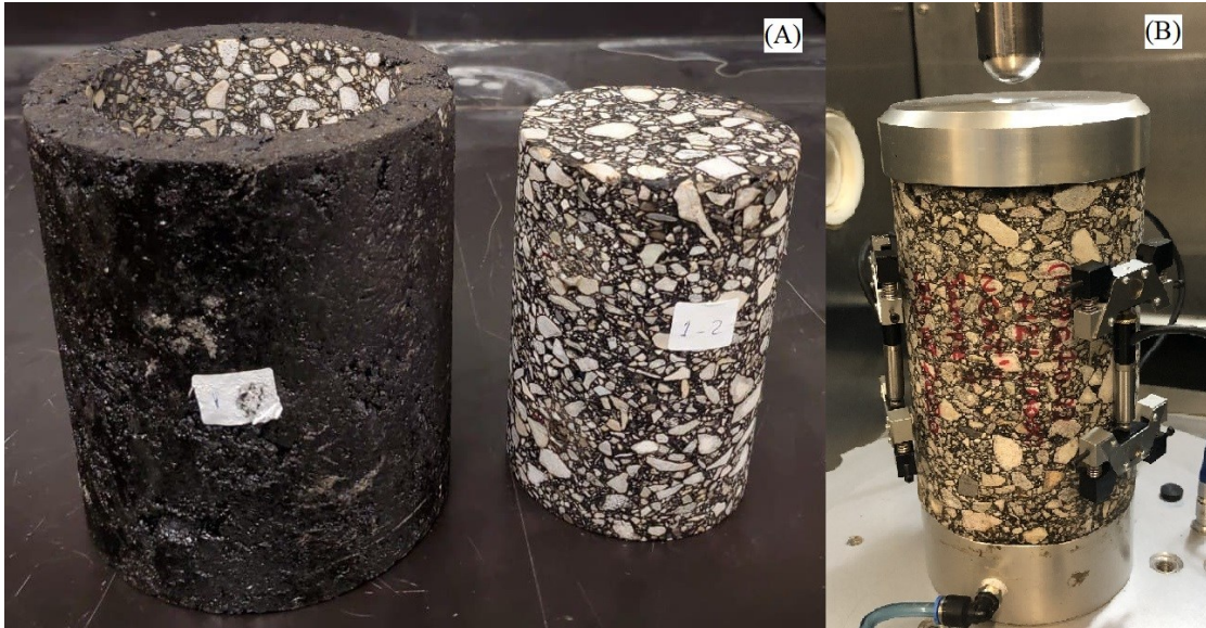
Figure 4: Cored and cut sample (A) dynamic modulus test setup (B)
