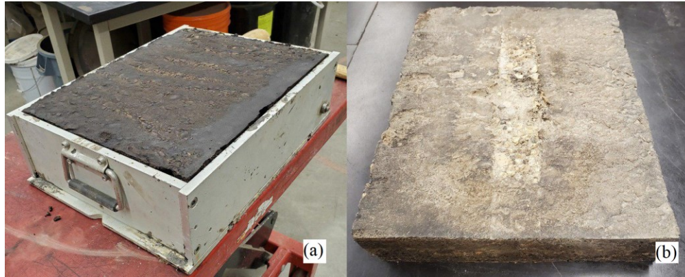
Figure 4-8 Slab samples compacted by roller compactor (a) prior and (b) after test
