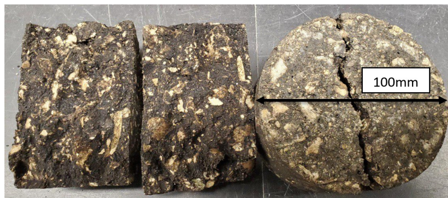
Figure 3-8 Compacted samples by Marshall hammer after performing ITS test
