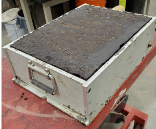
Figure 3-3 Slab sample compacted by roller compactor
