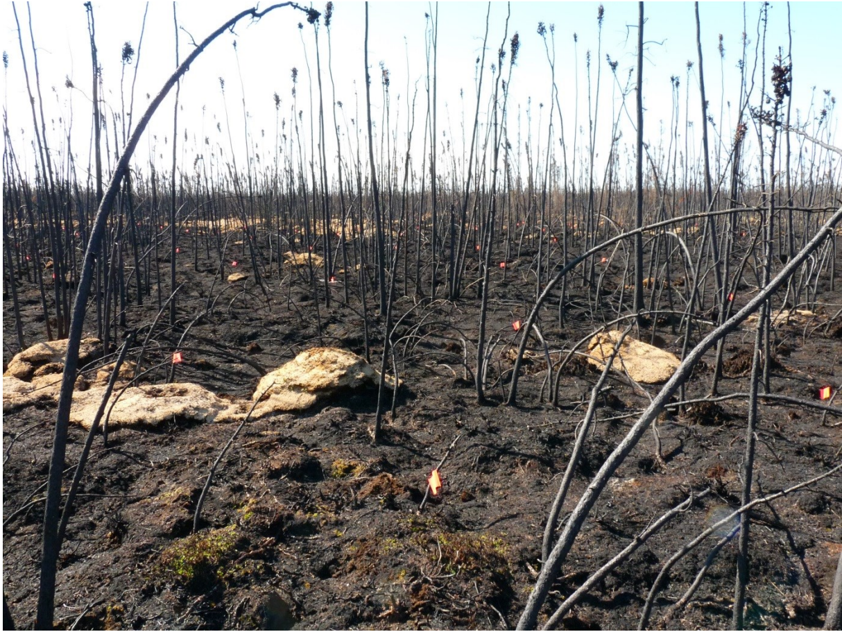
Figure S2.1. Example of a peat plateau site (Kakisa 2014) where soil thermal regime was monitored. Each peat plateau site had a 5 m spaced grid with 100 point locations marked with flags where depth to frost table was measured.
