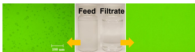
Figure 4. S7 Optical microscope images and digital photos of the SDS-stabilized hexane-in-water emulsion before and after separation.
