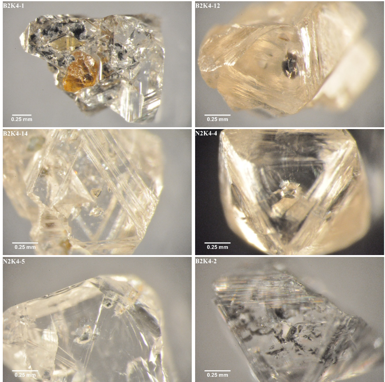
Figure B.5.1. Examples of inclusions within diamonds: orange garnet (B2K4-1), sulphide surrounded by fracture (B2K4-12), faint green clinopyroxenes (B2K4-14), colourless olivine (N2K4-4), mineral association of pale green clinopyroxene and orange garnet (N2K4-5) and graphite cluster (B2K4-2).
