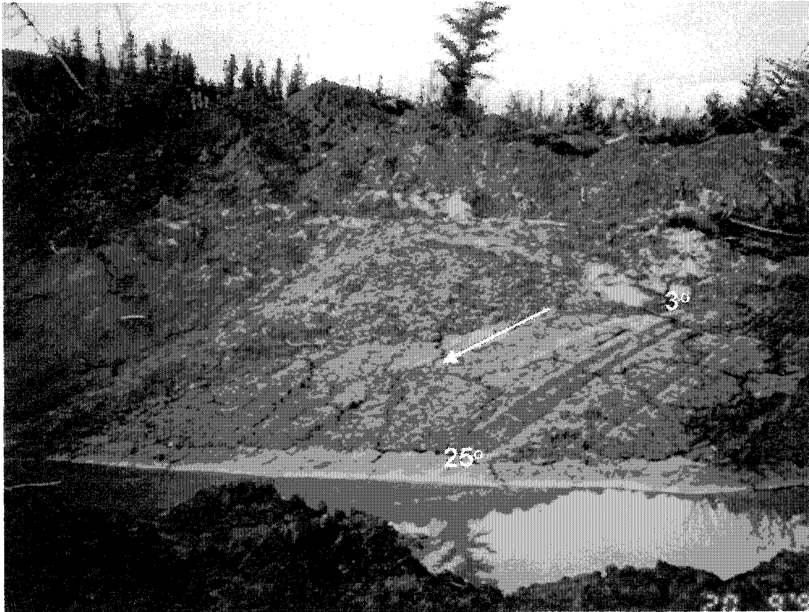
Figure 3.8 A convex rupture surface at site 36 (same as vane shear site E), at the toe of the rupture surface, separating the zone of depletion from the zone of accumulation. Note the pronounced striated slickensides. Bedding is at 3^\circ and the surface of rupture here has cut across the bedding.
