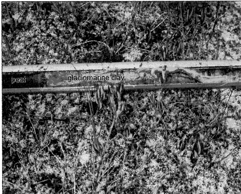
Figure 7.5 A Hiller peat corer showing the marine clay – peat interface. I sampled peat at these contacts to obtain minimum ages for the landslides.
