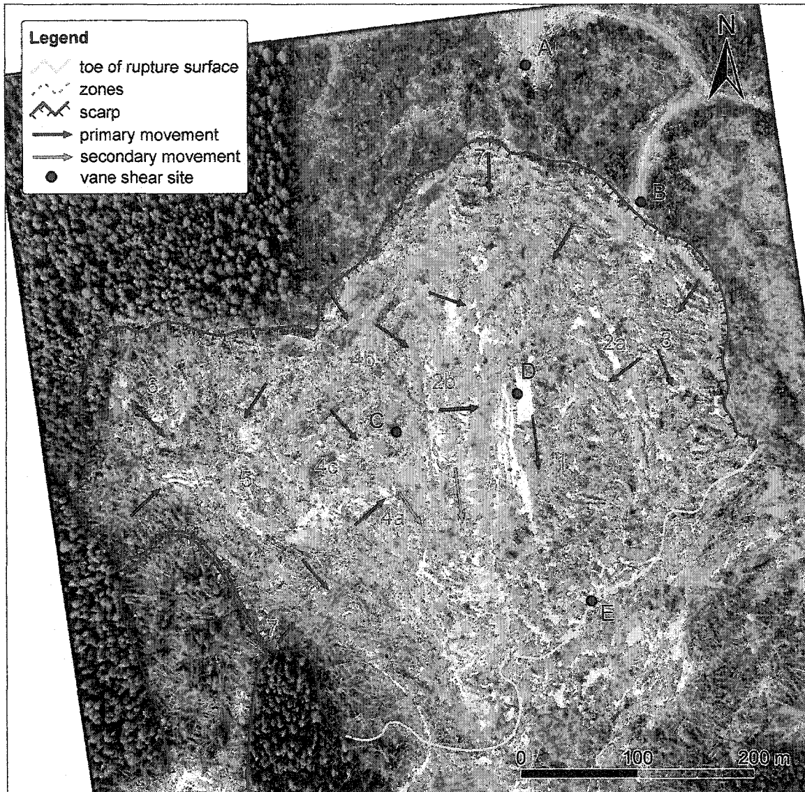
Figure 6.1 1994 orthophoto of the Mink Creek flowslide. Note the numbered zones distinguished on the basis of morphology and style and direction of movement (Chapter 3). The landslide to the southwest is separate from the main landslide. Red and blue arrows indicate direction of primary and secondary movements, respectively.
