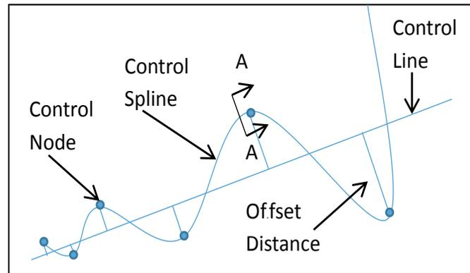
Figure 2.5: An example of parameterization for a center line. This is a plan view approximately 100s of meters in extent.
