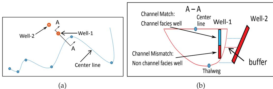
Figure 3.4: The calculation of the variables in the objective function. (a) A plan view displaying a well building its cross section view. (b) A cross section (NTS) showing the definition of variables in the objective function. The functions representing object boundary are already parameterized (Figure 2.10).
