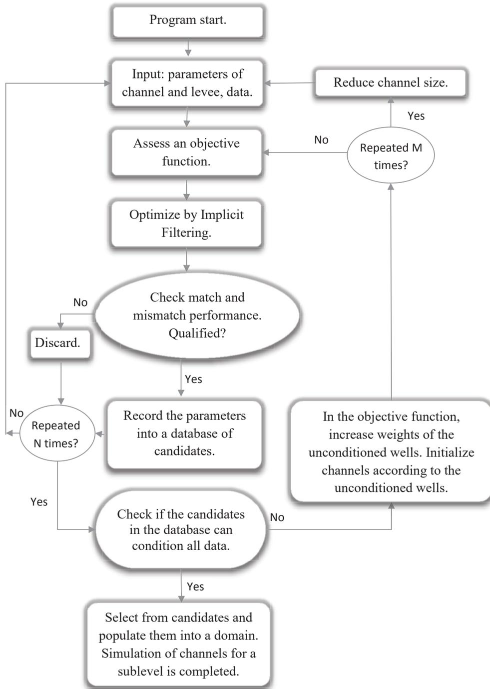
Figure 3.1: The work flow for simulation of single-type objects.
