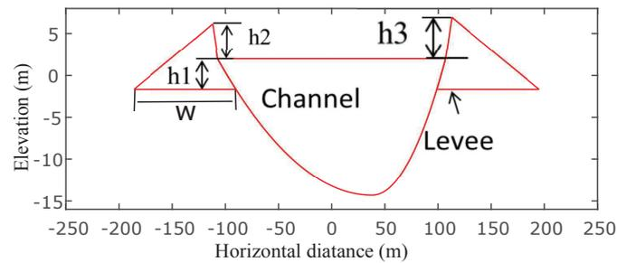
Figure 2.11: A cross section of a levee illustrating the parameterization. The X axis represents the horizontal distance on the cross section.
