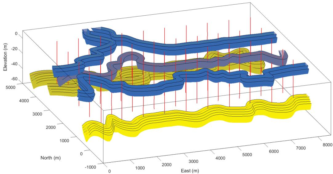
Figure 4.6: A reservoir constructed using the centerlines initialized according to well data. The non-channel wells (in red) are avoided by the channels. The channels are half transparent. The red wells transferring into blue wells can be seen at the top surface of channels. The blue wells transfer back to red wells at the bottom surface of the channels.
