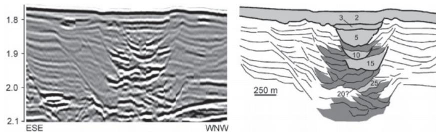
Figure 2.3: Channel profiles interpreted from seismic data (Deptuck et al., 2007). The left one is uninterpreted and the right one is interpreted.
