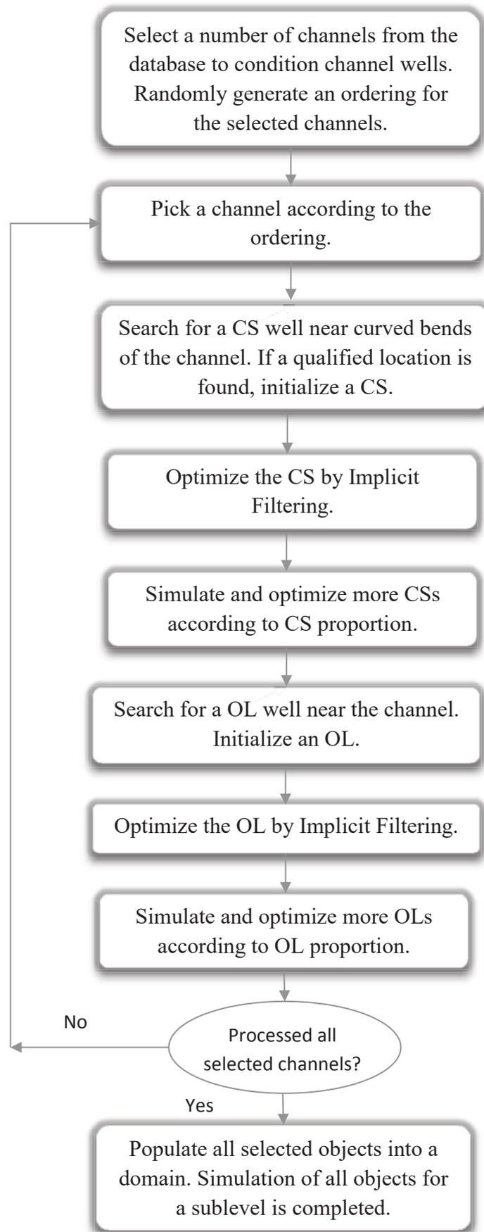
Figure 3.2: The work flow for simulation of one realization with all types of objects.
