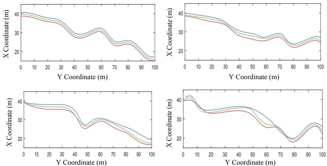
Figure 2.13: Center lines of stacking patterns (three elements represented by three colors). From left to right, top to bottom, the level of disorganization is increasing. The control variable is 0, 1/3, 2/3 and 1 respectively.
