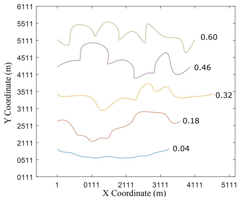
Figure 2.9: Centerlines generated with different amplitude:wavelength ratios, being 0.04, 0.18, 0.32, 0.46 and 0.6 respectively from bottom to top.
