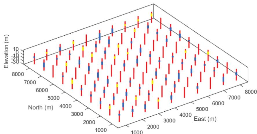
Figure 3.3: An example of well data. Red indicates floodplain facies, blue indicates channel and yellow indicates levee.
