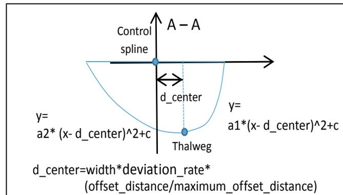
Figure 2.10: A channel profile (NTS) illustrating the parameterization.
