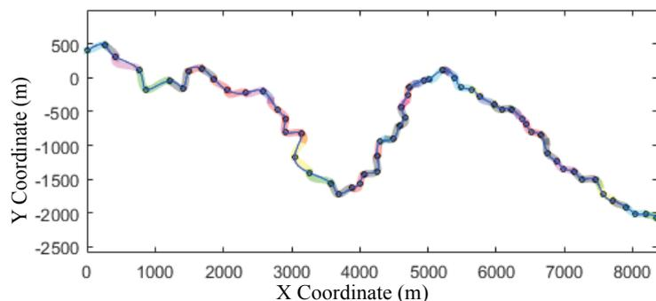
Figure 2.8: A centerline (the blue line) reproduced by interpolation of control nodes. In comparison, the colorful lines are the original centerline.
