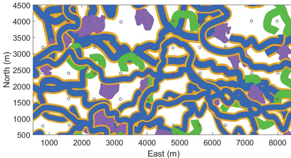
Figure 3.13: A simulation with all objects conditioned to well data. The square, cross, circle, diamond and star represent channel, levee, floodplain, crevasse splay and oxbow lake facies well respectively.
