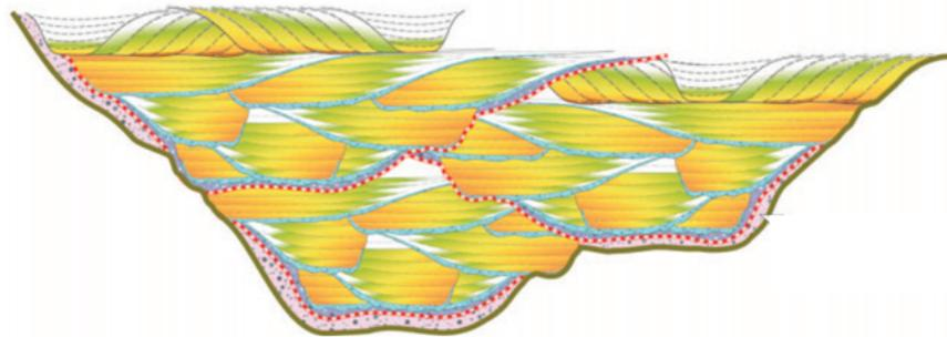
Figure 2.1: Hierarchy of a channel complex (Alpak et al., 2013). This cross section represents a thickness of 50-200 m and a width of 800-4000 m.
