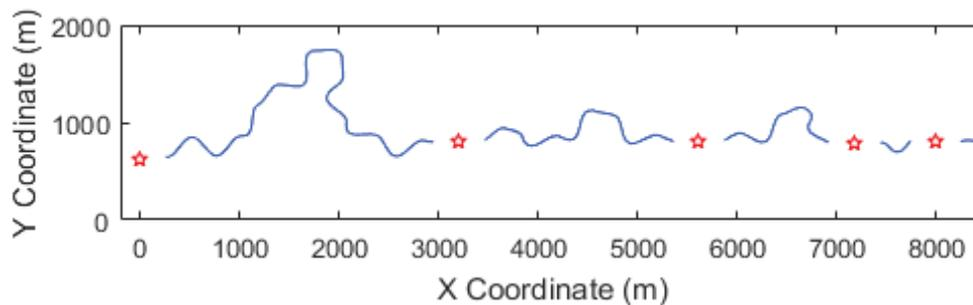
Figure 4.5: A centerline initialized according to well data. Red stars indicate the wells and blue lines are the centerline segments passing near the wells.
