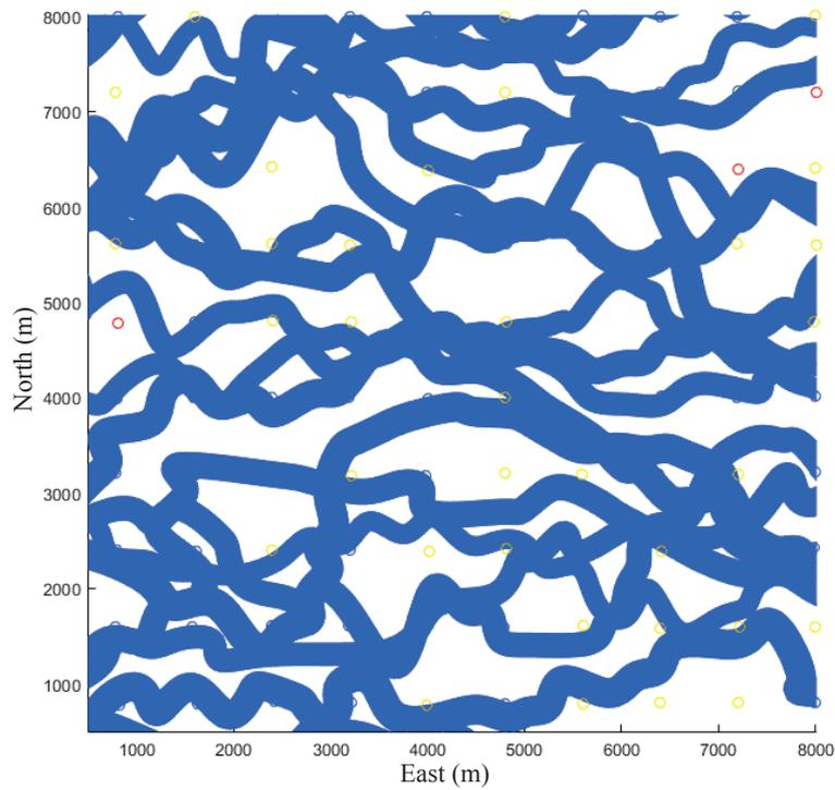
Figure 3.9: A plan view for a realization with relatively-dense data. Channel wells are in blue and are covered by channels. Non-channel wells are in red and are avoided by channels. Yellow levee wells are not conditioned in this example.
