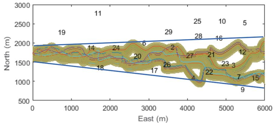
Figure 4.12: Modeling of 1D horizontal trend. The two blue lines represent the range of channels. There is an obvious proportion trend from left to right. Each number in the middle of the figure represents a well. Every channel well is conditioned.
