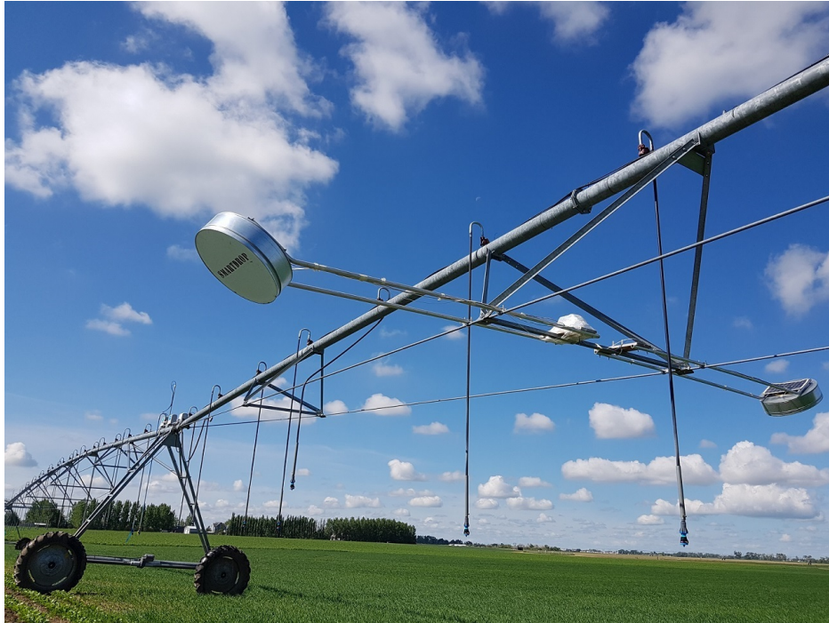
Figure 3.1: Microwave remote sensors on a central pivot.
