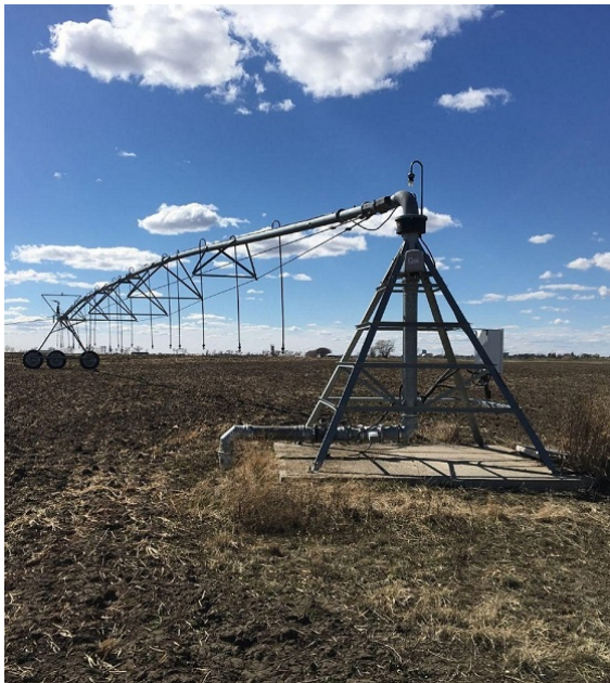
(a) The center pivot irrigation system of the field.
