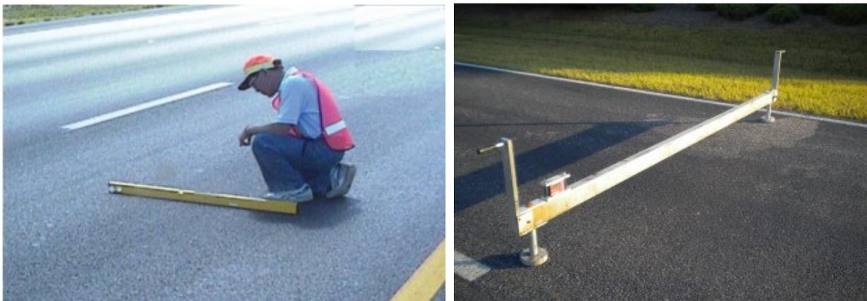
*Figure 13: Road Slope Measurements Using Digital Level*
