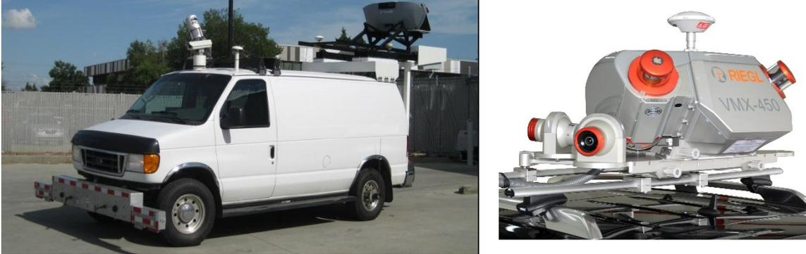
Figure 10: Multi-Function Pavement Surface Profiling Vehicle (Left), VMX-450 MLS System (Right).
