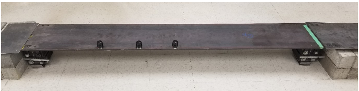
Figure 2-3: Pin-roller bridge setup.
