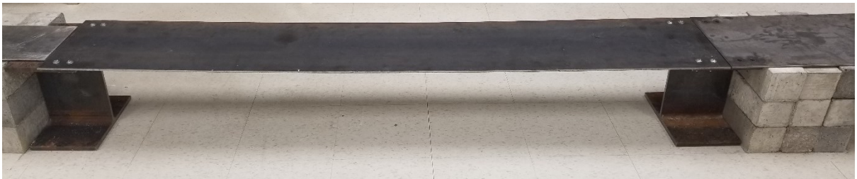
Figure 2-5: Fixed-fixed bridge setup.
