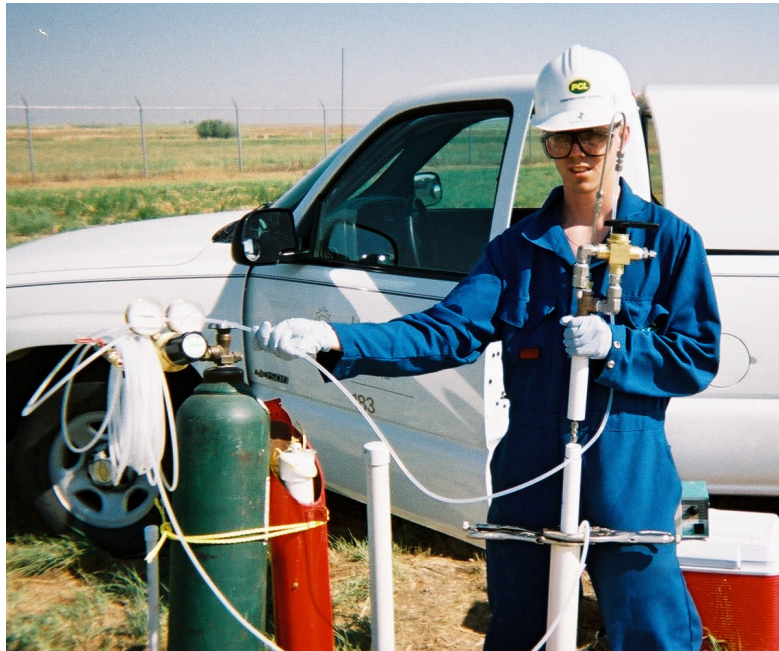
BarCad Sampling Method with Compressed Argon: P34 cluster
