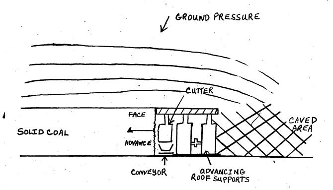
(ii) Because of its flexibility longwall equipment can be used in shallow seams measuring between 32 and 42 inches high. Conventional and continuous miners cannot be used in such seams and there will be a greater shift to longwall as more seams of this height come into production in the future.
