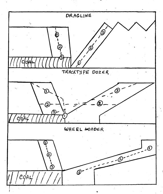
overburden from this initial cut, or trench, is deposited on the outskirts of the mining area. When the coal has been removed from this first trench, a second cut is made parallel to the first with the overburden of this second trench deposited in the first. This operation is continued until the boundary of the mineable region is reached. Furrows and mounds are found throughout the entire mining region but these are easily leveled by a bulldozer.
