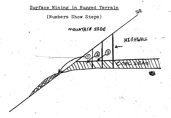
Contour mining is very similar but, as its name implies, the various trenches occur in a circular fashion as the mining equipment proceeds all the way around an uplifted area. In this case the coal seam usually underlies the entire uplifted area (or mountain).
