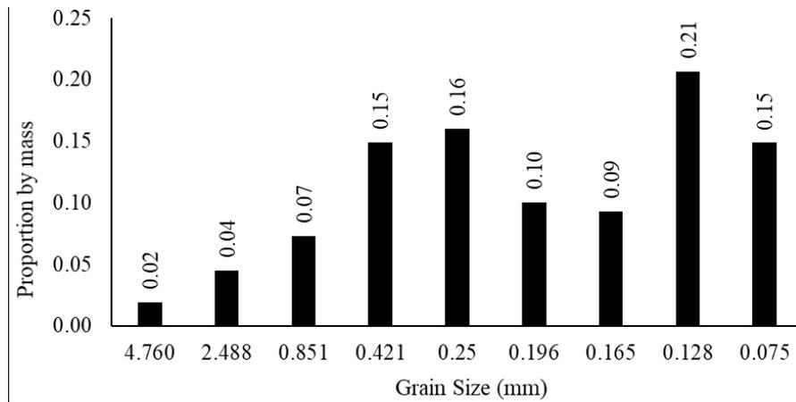
Figure 8.3 Particle size classes used in CAESAR-Lisflood simulations.
