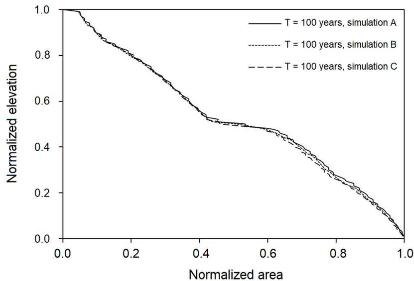
*Figure 9.9 Hypsometric curves for the dam section for all simulations after 100 years*
