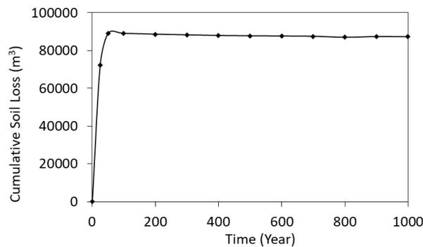
Figure 8.10 Soil loss from the dam (soil eroded from the slope) over 1000 years.
