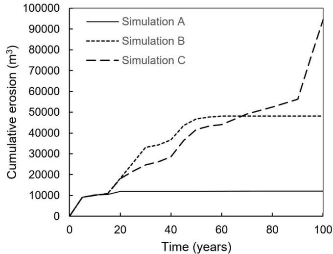
Figure 9.11 Cumulative soil loss (eroded volume) from dam slope over 100 years of simulation.
