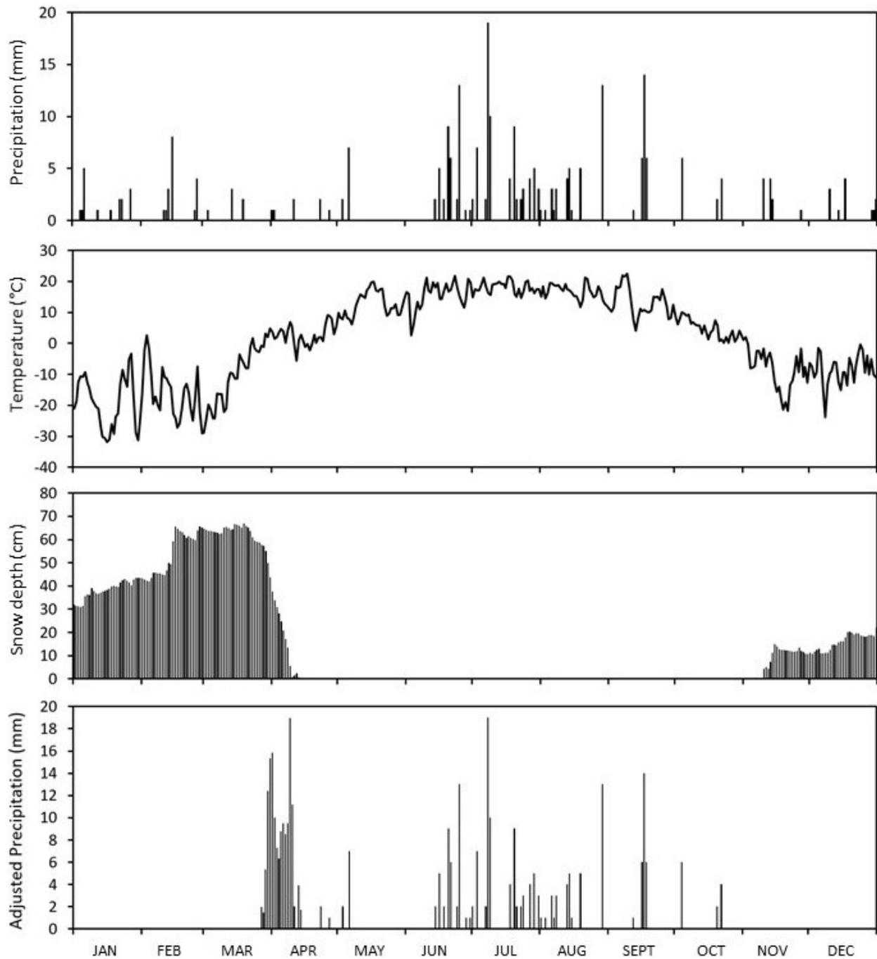
Figure 8.4 Illustration of precipitation data adjustment for winter conditions and snow melt. The adjusted precipitation was input to CAESAR-Lisflood for simulations.
