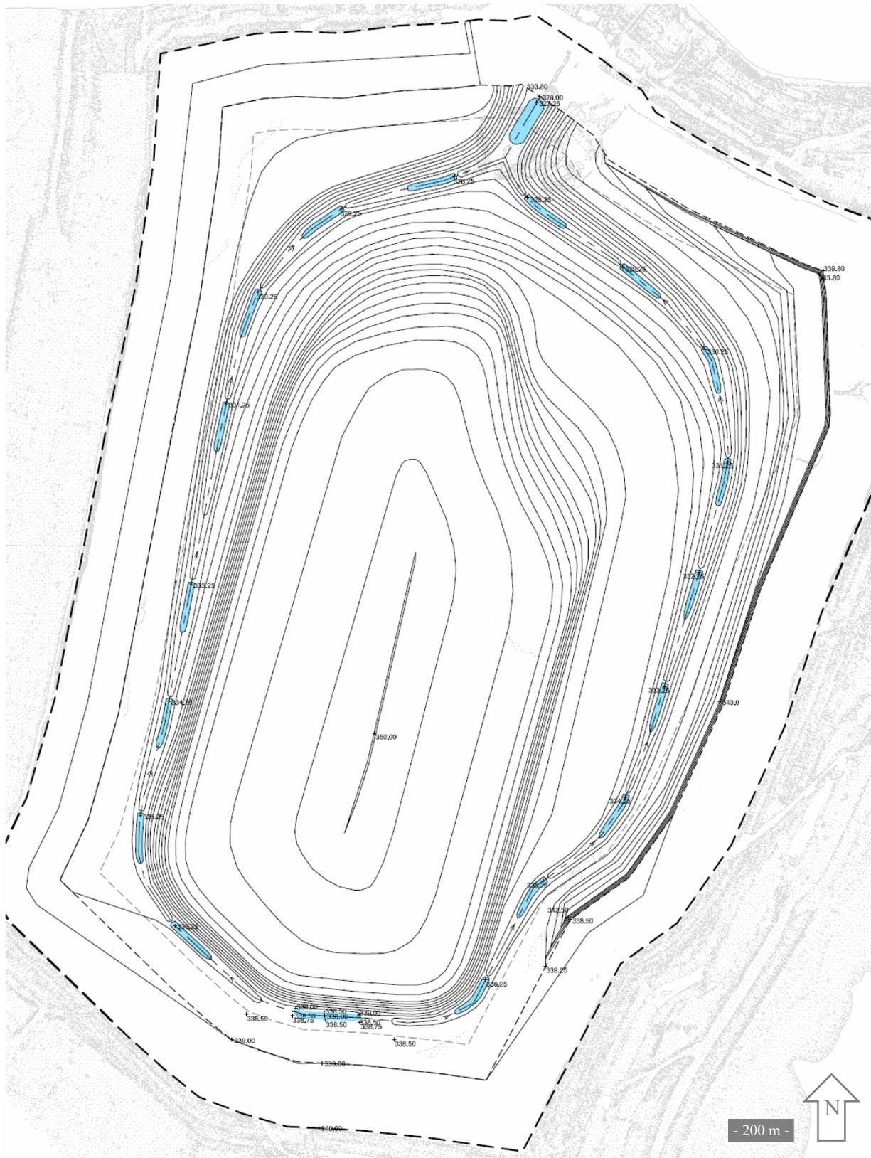
Figure 3.14 Tailings storage facility closure topographic design Option 'C': "Dome". Volume maximization using 15% maximum slope.
