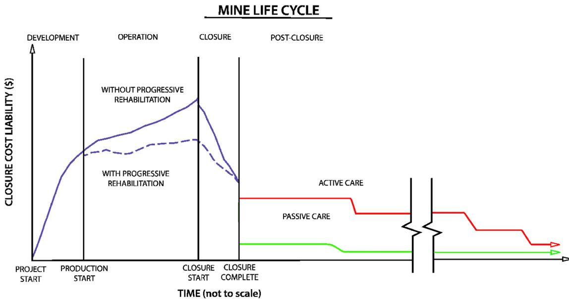
Figure 2.5 Closure cost liability with and without progressive reclamation. Bocking, 2010.
