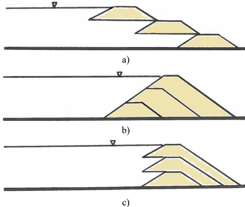
*Figure 2.2 Tailings dam construction types: (a) upstream, (b) downstream, and (c) centerline construction. Upstream construction is banned in many seismic regions.*
