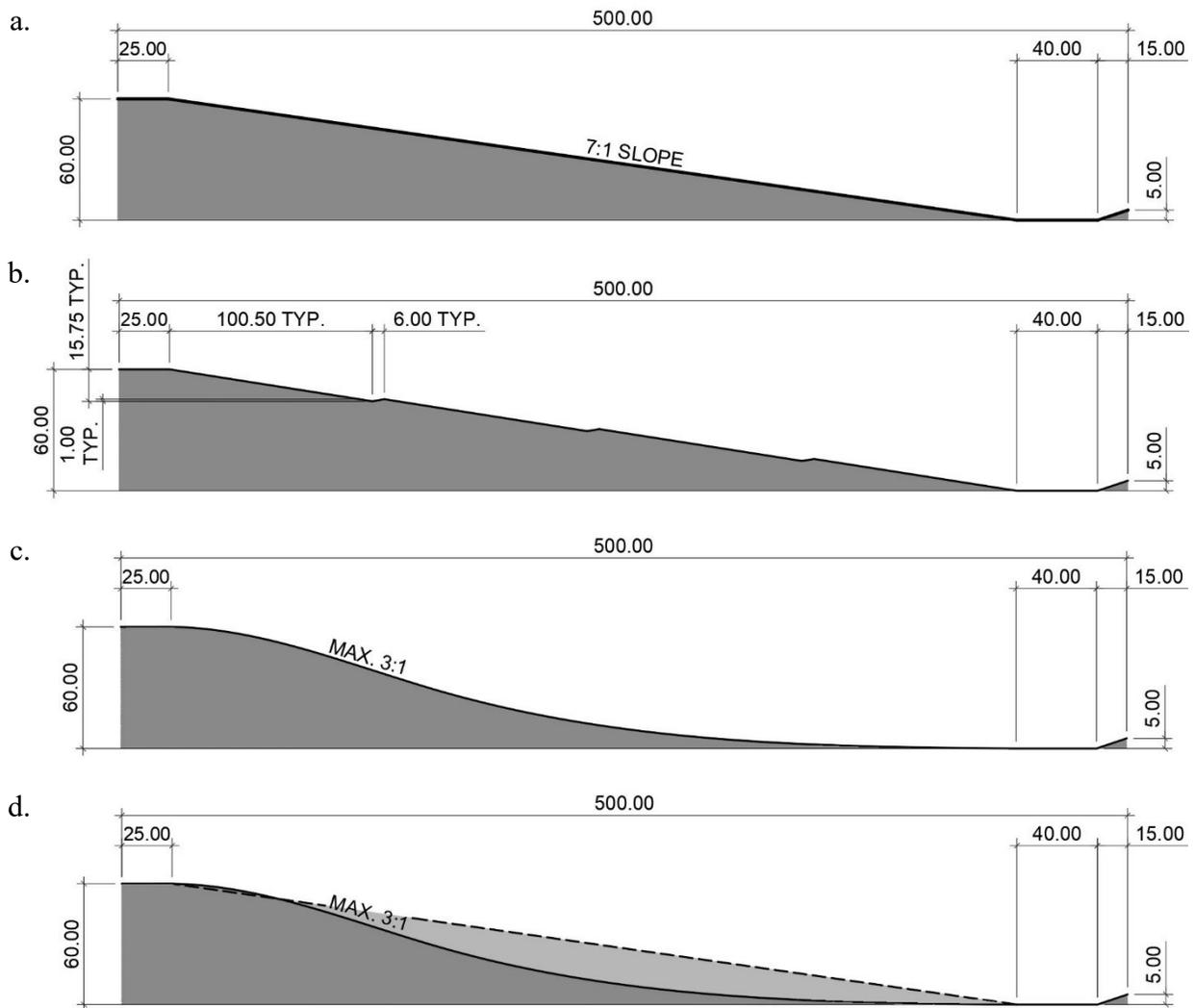
Figure 10.1 Cross-sections through centreline of dam designs: (a) constant slope, (b) platform-bank, (c) catena, (d) directed flow and armoured directed flow (with dashed line showing cross section at edges). All dimensions in meters, slopes H:V.
