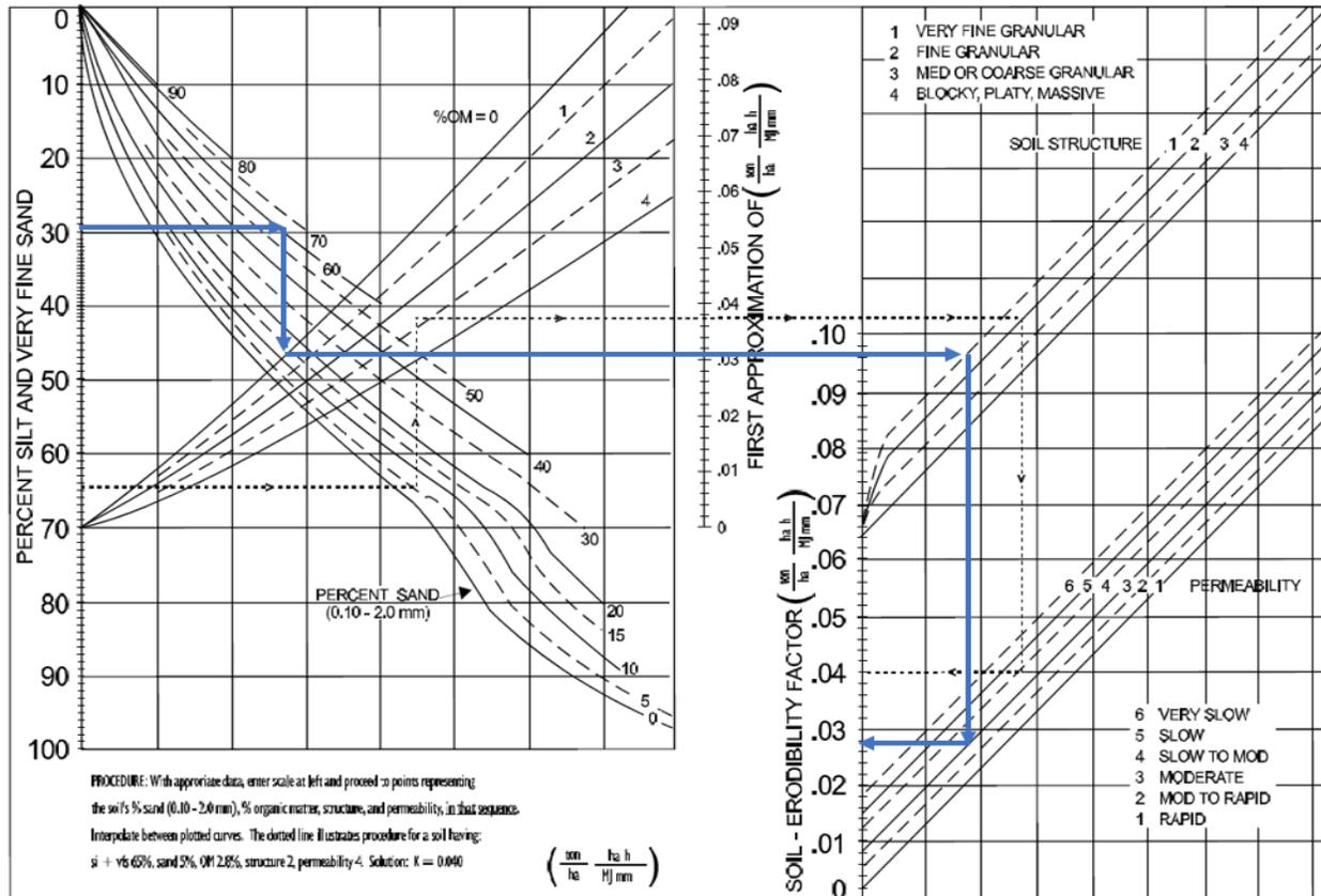
Figure 5.6 Nomograph for determination of  $K$ . In this case, for CST we find  $K = 0.027$ . From Wall et al., (2002).
