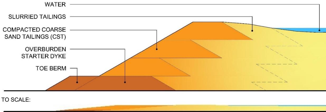
Figure 9.5 Hypothetical tailings dam cross section vertically exaggerated to illustrate the upstream construction method widely used in the AOS (top), and shown to scale below.
