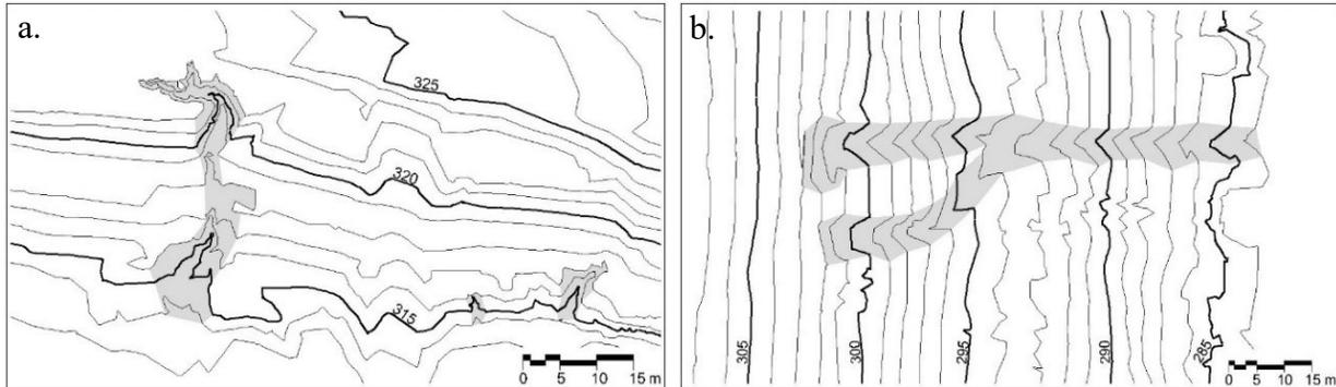
Figure 6.10 Gullies (shaded grey) identified through LiDAR analysis as viewed with a 1 m contour interval using AutoCAD. (a) On the left, pooled water caused the large gully here, while gullies shown in the right image (b) are caused by seepage.
