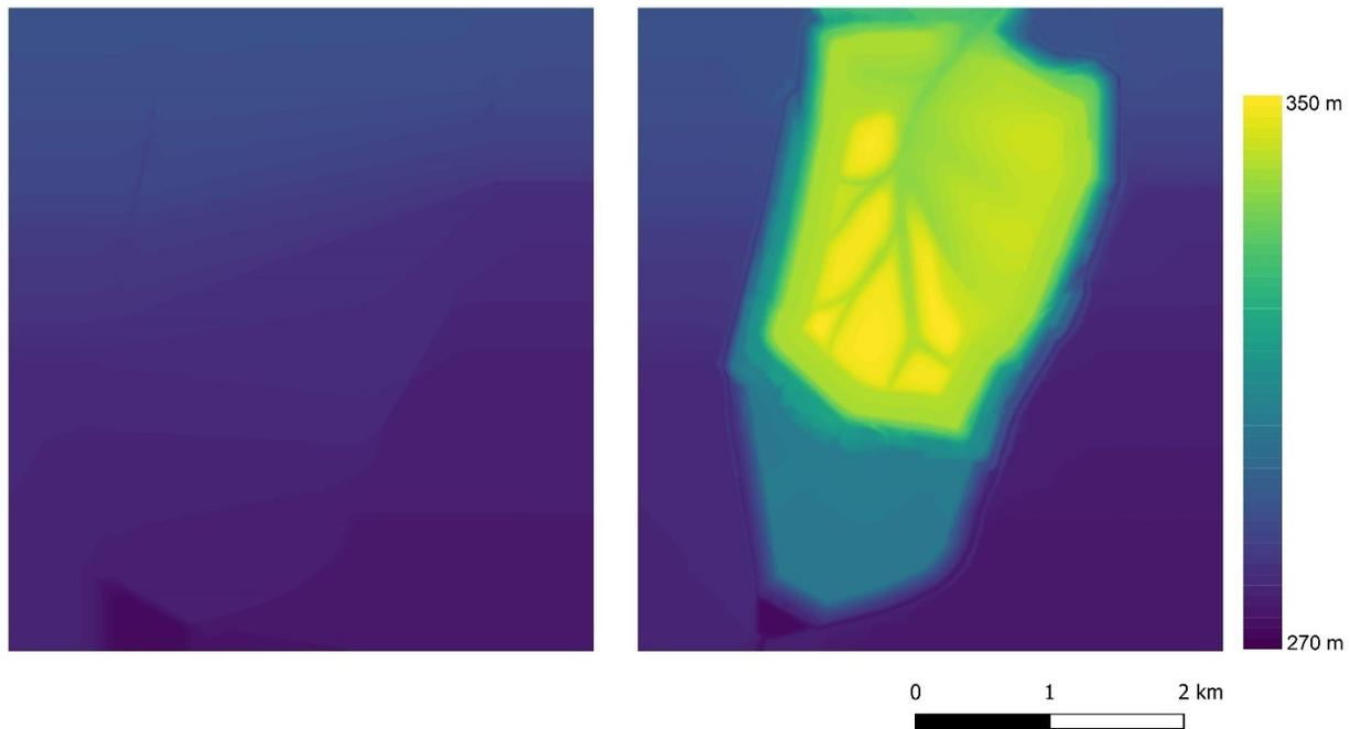
Figure 8.1 *Bedrock DEM (left) and surface topography DEM (right) used in the first simulation (200-years), both with north to the top of the page.*
