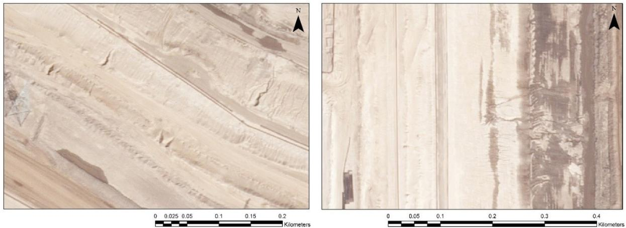
*Figure 6.11 Erosion features visible on digital aerial photography. Gullies and large areas of rills are visible on the left (a). Wind-blown CST appears light in colour and seepage generating gullies appears dark in colour on the right image (b).*
