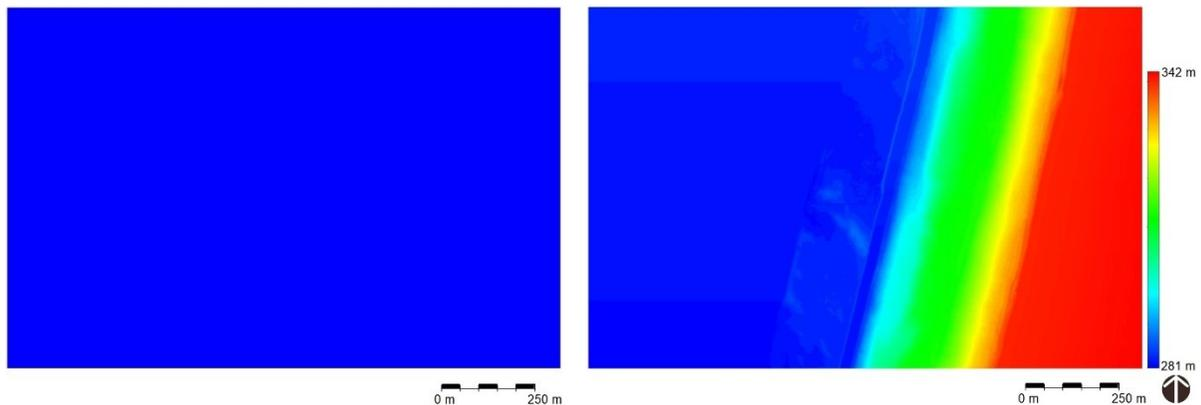
Figure 8.2 *Bedrock DEM (left) and surface topography DEM (right) used in 1000-year and 100-year simulations, both with a cell size of 2.5 m and dimensions of 592 x 386 cells.*
