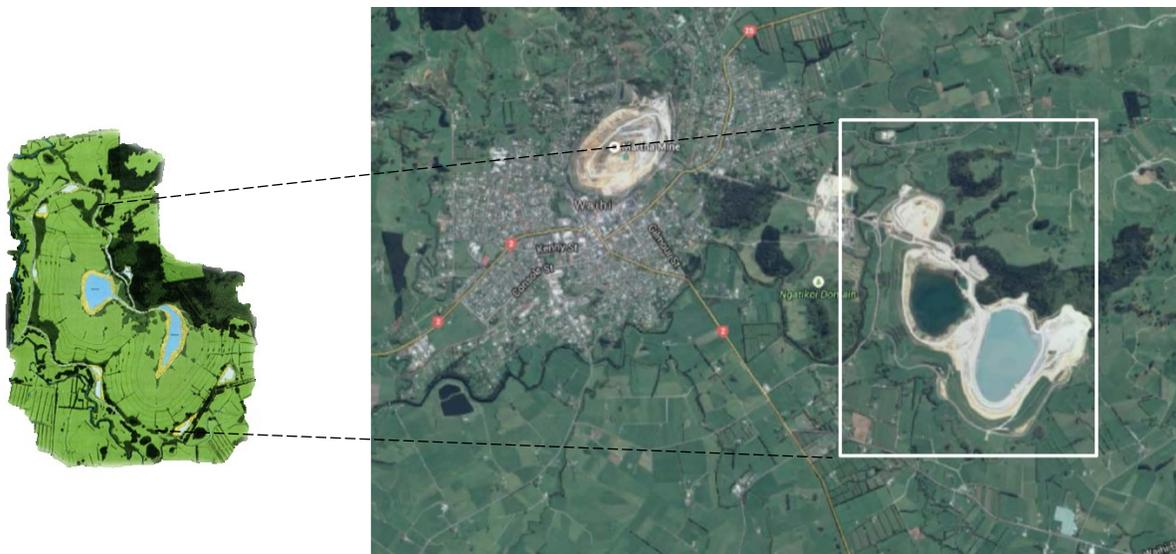
Figure 2.9 Concept plan for Waihi Gold Mine's waste rock embankments and tailings ponds (left), compared to aerial image of the site from 2015. (Concept plan from <http://www.waihigold.co.nz/environment/rehabilitation>, aerial image from google earth.)
