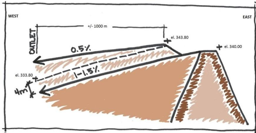
Figure 3.8 Schematic cross-section of north-east area of TSF. Outlet elevation and capping assumptions as shown. Note red wedge, loading fine materials on the west more than coarse materials on the east.
