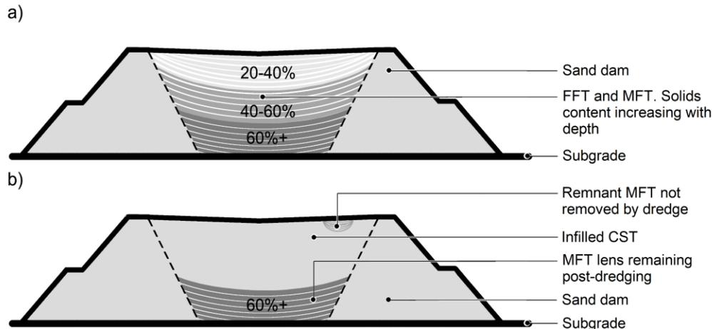
Figure 4.4 Schematic oil sands tailings dam composition a) after tailings deposition ceases and b) the same tailings dam after the pumpable portion of MFT is removed and infilled with coarse sand tailings
