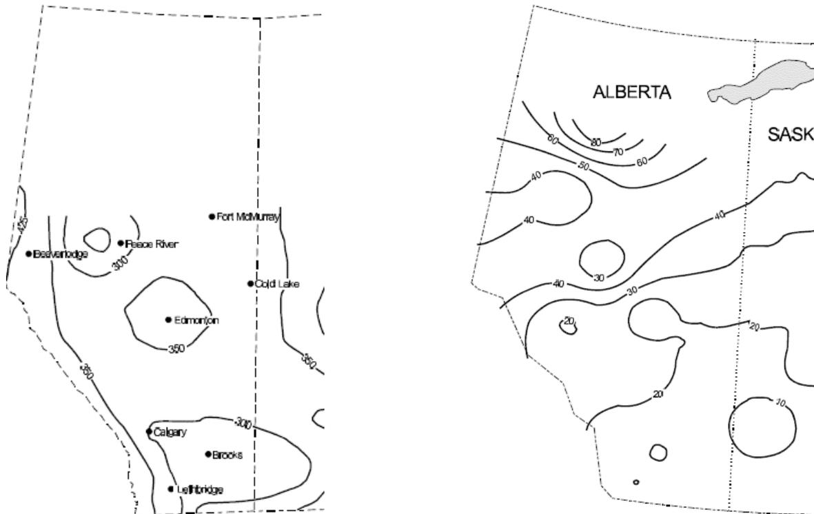
Figure 5.5 (a) Isoerodent map for Alberta showing  $R$  values (left), and (b) adjustment value,  $R_s$ , for winter conditions in Alberta (right). Note Ft. McMurray,  $R = 325$  and  $R_s = 40$ , therefore  $R_t = 365$ . Isoerodent maps edited for clarity from Wall et al. (2002).
