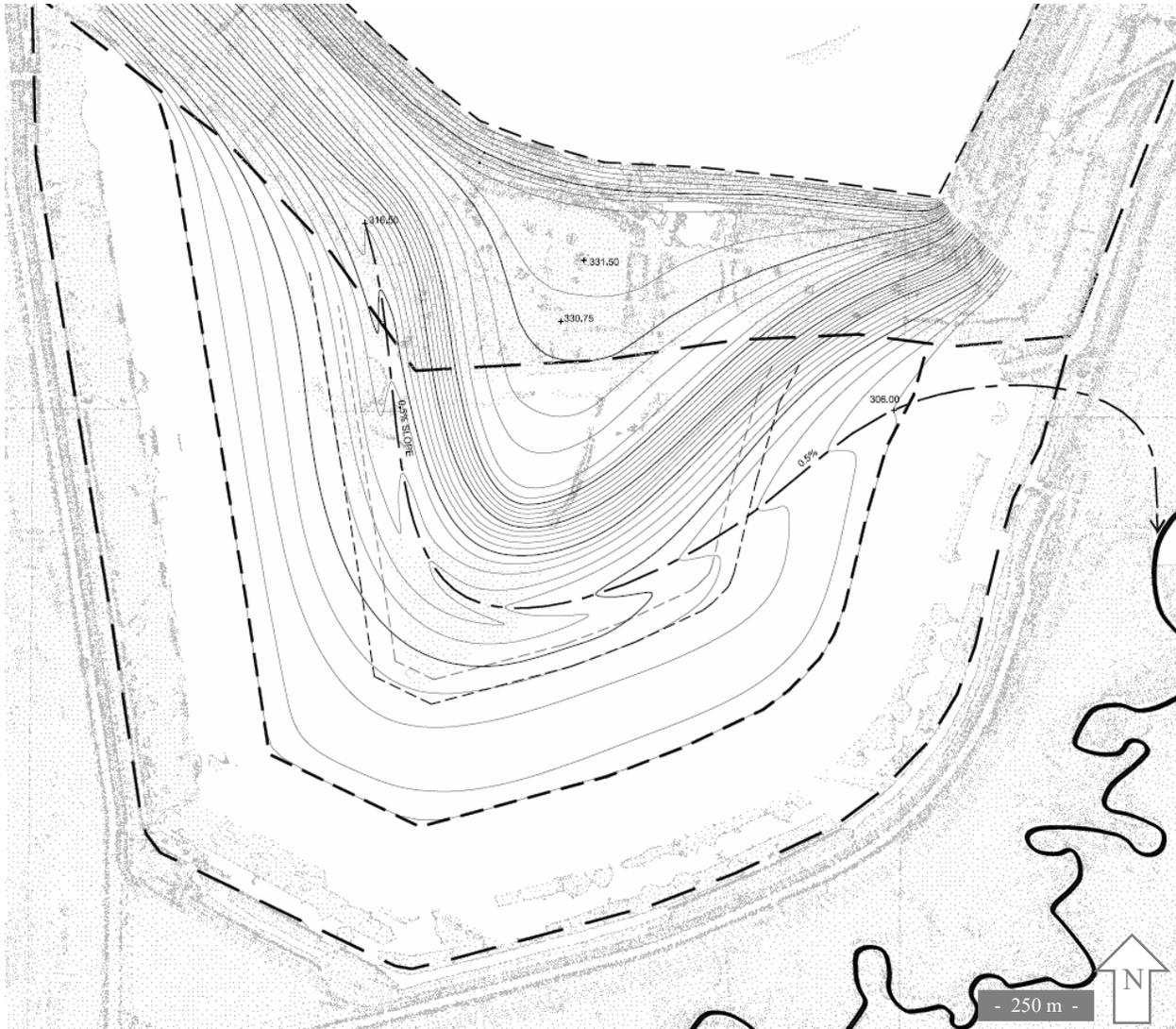
Figure 3.17 South expansion area closure topographic design Option 'Three'.
