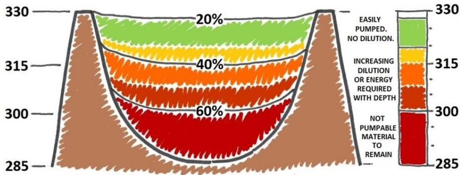
Figure 3.6 Sketch of solids content with depth in the TSF. As % solids of FFT pumped increase, the post-dilution volume increases, as do the associated time to pump and space requirements for one unit of pre-diluted material. Data from Esposito and Nik, 2012.
