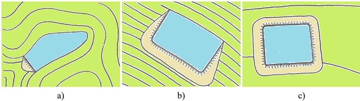
Figure 2.1 Tailings dam layouts: a) valley-fill or “cross-valley”, b) Side-hill, and c) ring-dyke.
