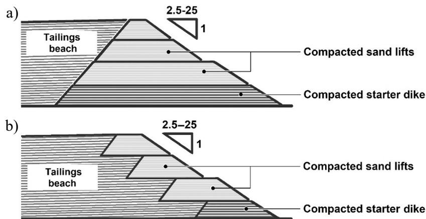
Figure 4.3 a) Common modified centerline and b) upstream tailings dam construction used in the Athabasca Oil Sands. Starter dykes are often constructed of lean oil sands, while each layer above is typically hydraulically placed, then mechanically compacted coarse sand tailings. Both sketches are vertically exaggerated and not to scale.
