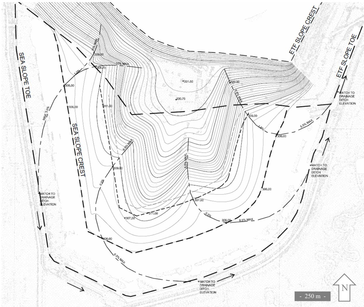
Figure 3.15 South expansion area closure topographic design Option 'One'
