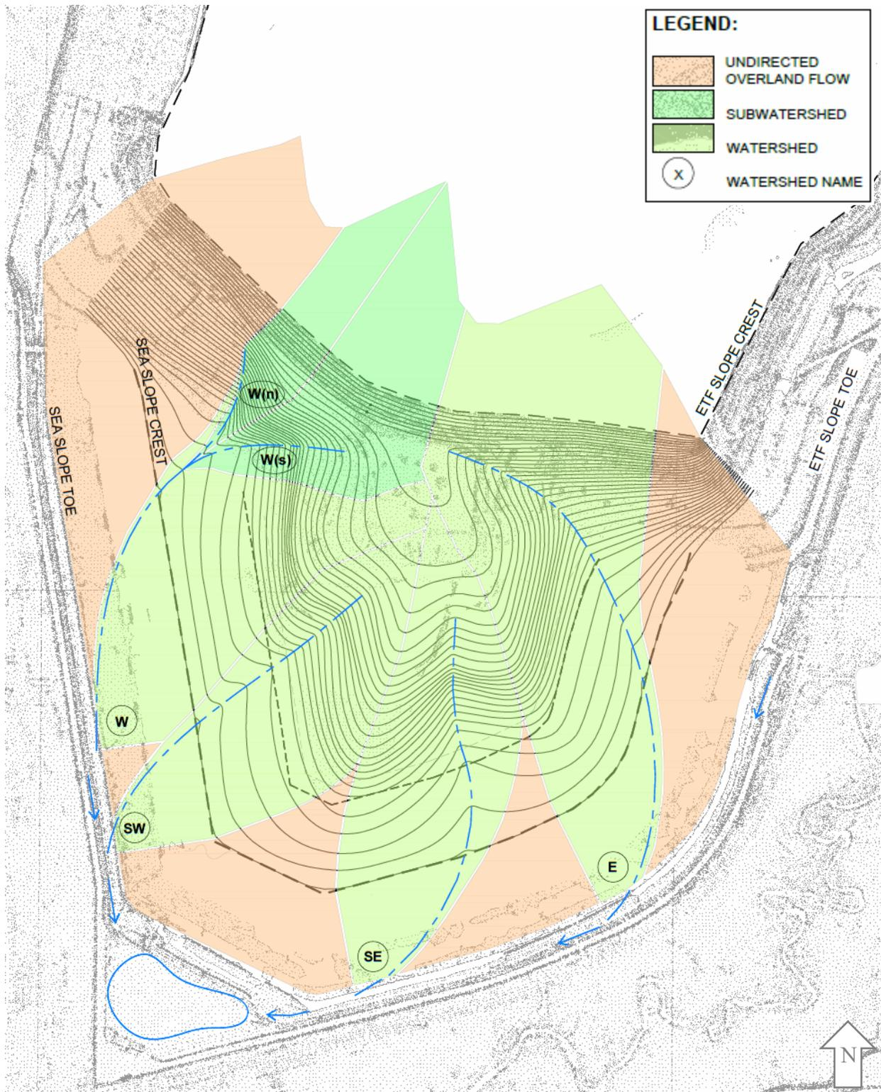
Figure A.5 Drainage Basins designed for the SEA Closure Topographic Design Option 'Two'.
