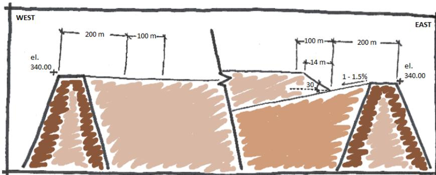
Figure 3.7 Minimum offsets from downstream crest, and capping/infill heights.
