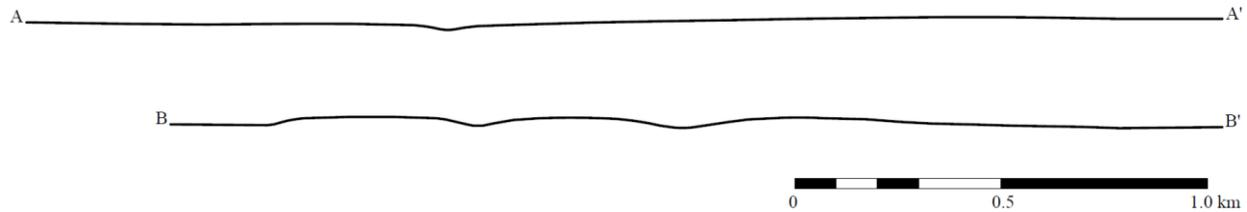
Figure 3.19 Cross sections A-A' and B-B' through geomorphically designed preferred closure topographic and drainage design (as noted in Figure 3.18). 3x vertical exaggeration.
