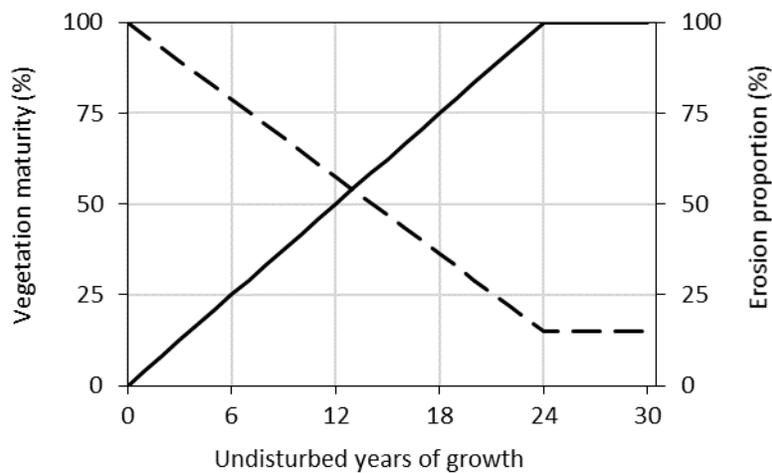
Figure 7.2 Relationship between vegetation maturity (solid line) and corresponding proportion of erosion (dashed line) permitted to occur. Adapted from Slingerland et al., 2018.
