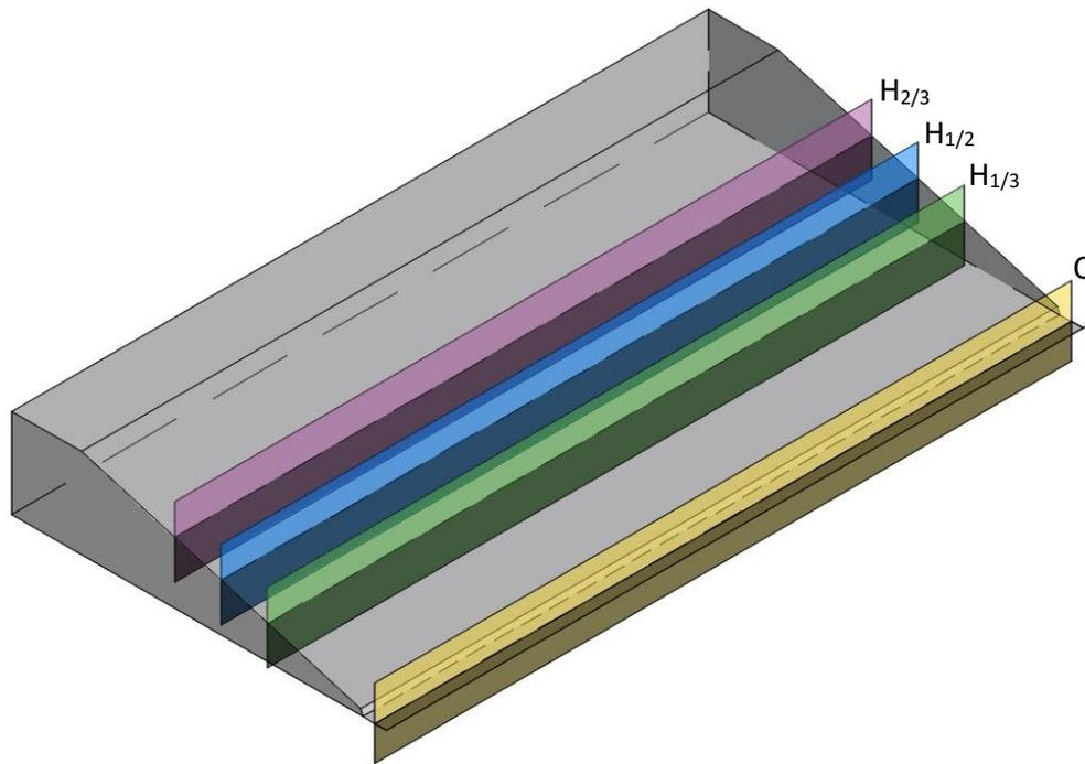
Figure 9.7 Locations of sections through the downstream face of a roughly 1 km section of the tailings dam, as illustrated in Figure 9.8.
