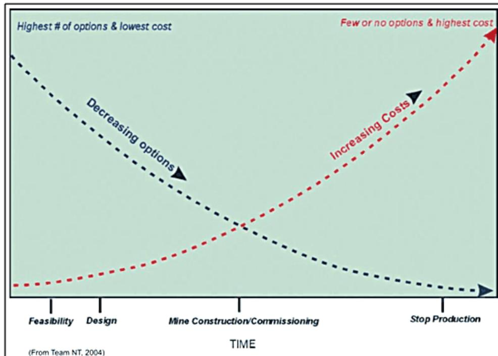
Figure 2.4 Acid rock drainage mitigation options and costs over the mine life. From the GARD Guide (INAP, 2009)
