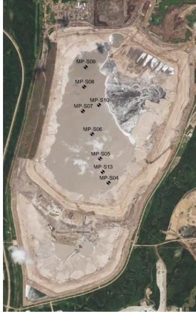
Figure 3.5 Sampling locations corresponding to greatest expected MFT depth to remain following infilling. From Esposito and Nik, 2012.
