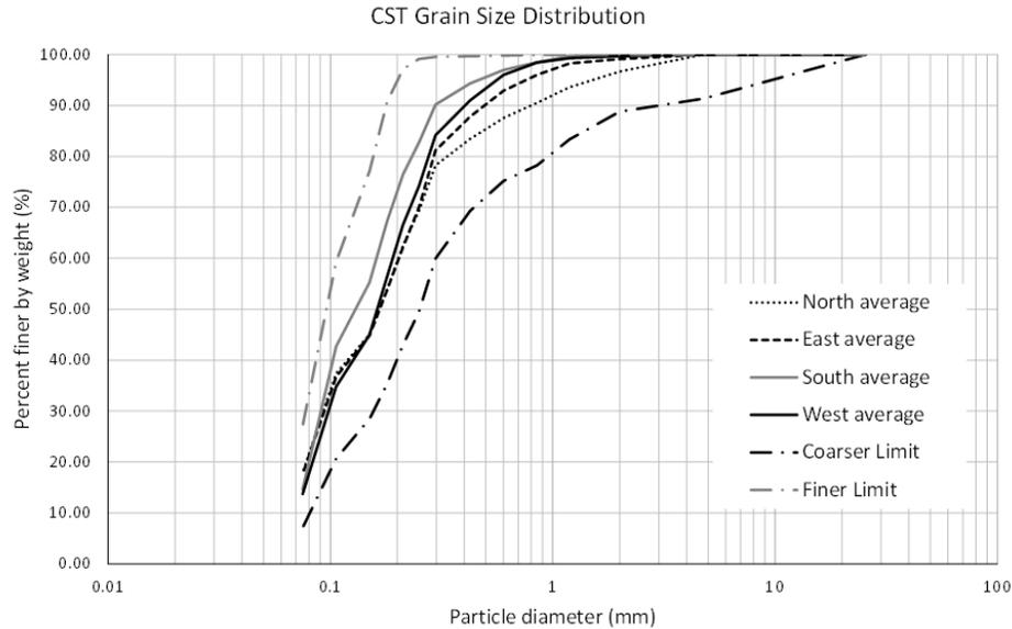
Figure 6.4 Grain size distributions of surficial CST collected from downstream dam slopes.
