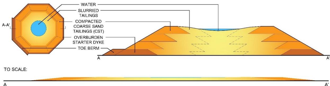
Figure 2.3 Fictional TSF in plan view (left) and section (right) at approximately 10x vertical exaggeration. Drawings not to scale. TSF cross section drawn to scale below.
