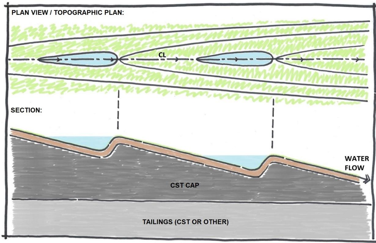
Figure 3.10 Ephemeral pools designed to slow water flow. Sketch is vertically exaggerated (in section) and has not been drawn to scale. Layer above CST is reclamation material consisting of a minimum 0.5m depth of peat mineral mix.
