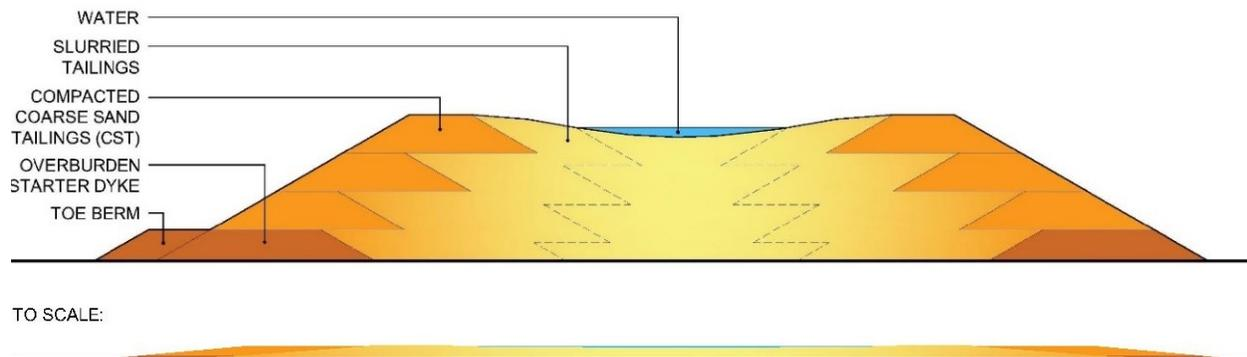
Figure 6.2 Upstream tailings dam construction in the oil sands. Shown to scale on bottom. Adapted from Slingerland, Beier, & Wilson (2018).
