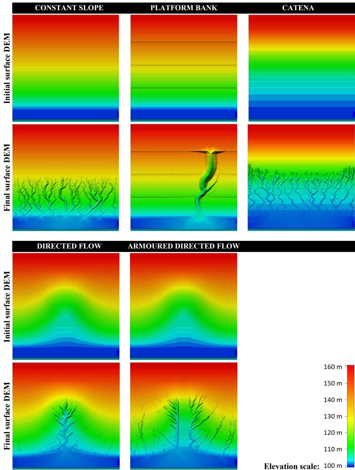
Figure 10.4 Initial and final DEMs illustrating the five dam surface designs. Each DEM has dimensions of 500 x 500 m.
