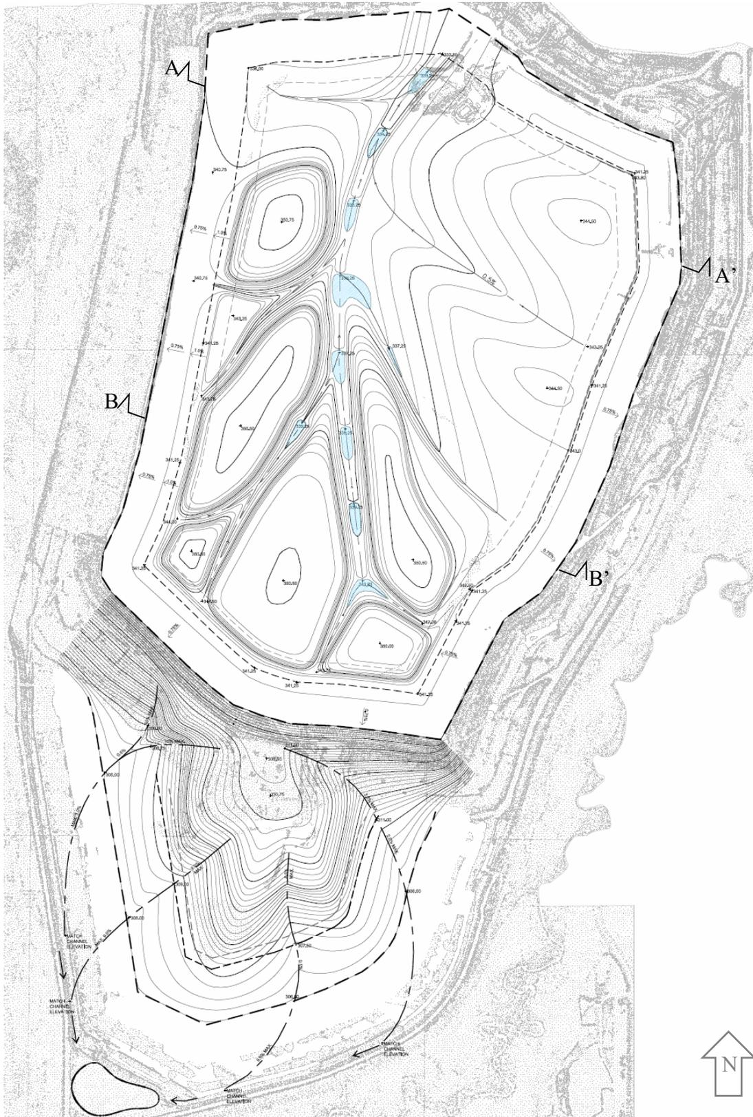
Figure 3.18 TSF and SEA preferred closure topographic and drainage design. See Figure 3.19 for indicated surficial cross sections. Drawing not to scale.
