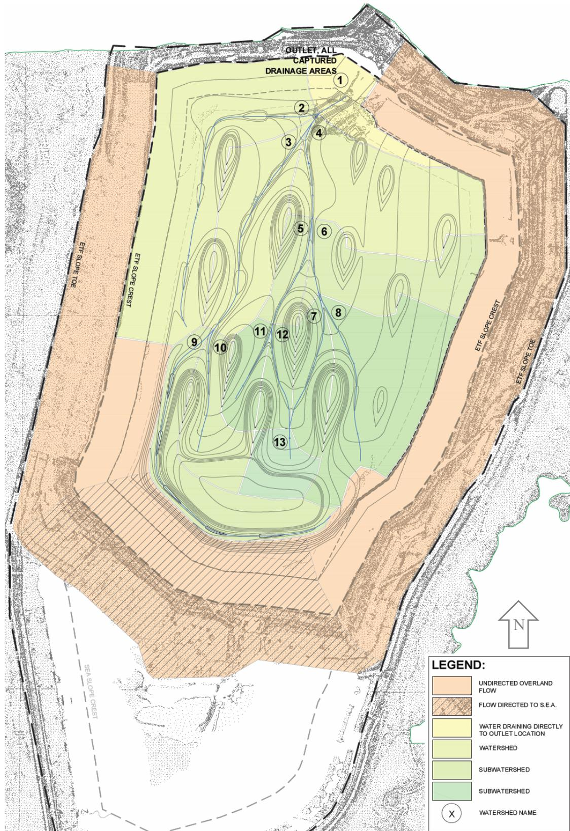
Figure A.1 Drainage Basins designed for the TSF Closure Topographic Design Option 'A' - "Drumlins".
