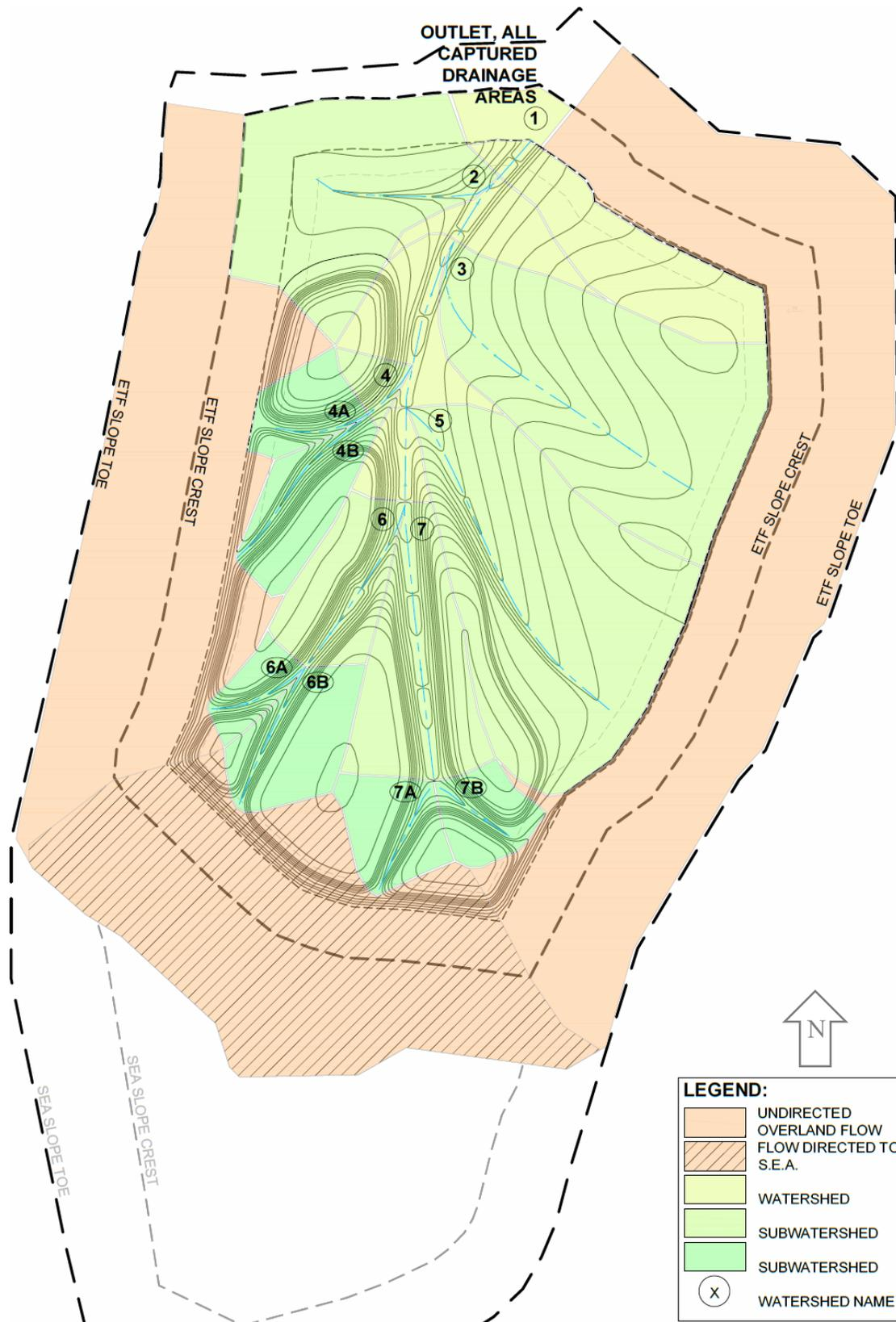
Figure A.2 Drainage Basins designed for the TSF Closure Topographic Design Option 'B' - "Ridge and Swale".
