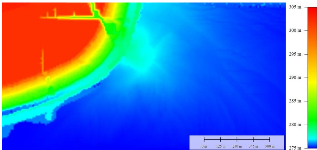
Figure 8.13 DEM following 200 years of simulation. A gully in the upper left has eroded the dam and deposited CST in a fan extending to the lower right corner of the image.
