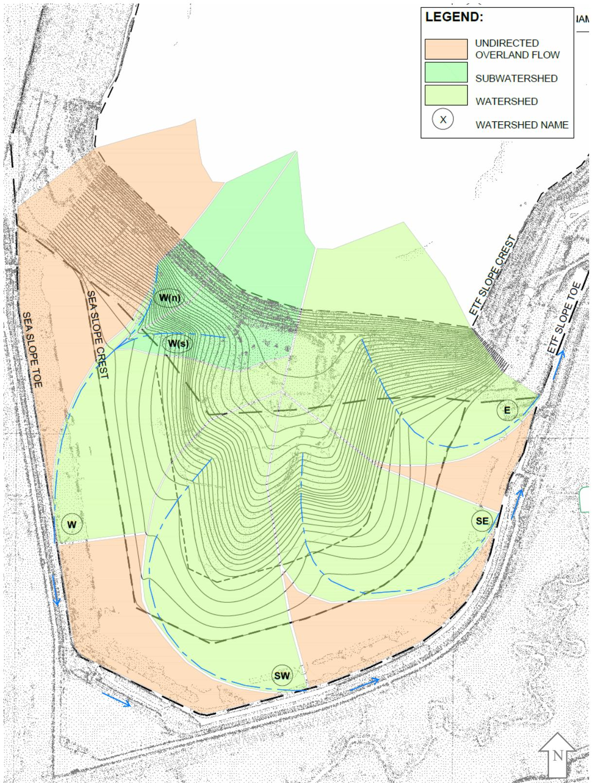
Figure A.4 Drainage Basins designed for the SEA Closure Topographic Design Option 'One'.
