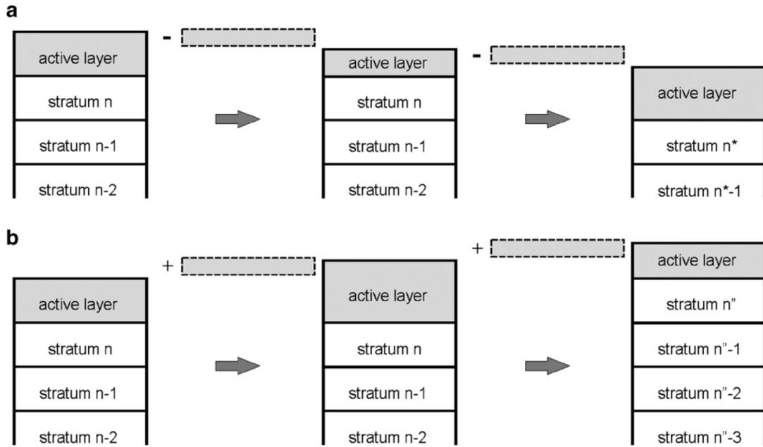
Figure 7.1 Illustrated changes to the active layer via (a) erosion and (b) deposition. Stratum layers are named according to their distance from the active layer: during erosion when stratum  $n$  becomes the new active layer,  $n-1$  becomes  $n^*$ , etc. and during deposition when the active layer becomes stratum  $n''$ ,  $n$  becomes  $n''-1$ , etc. From Van de Wiel, Coulthard, Macklin, & Lewin, 2007.
