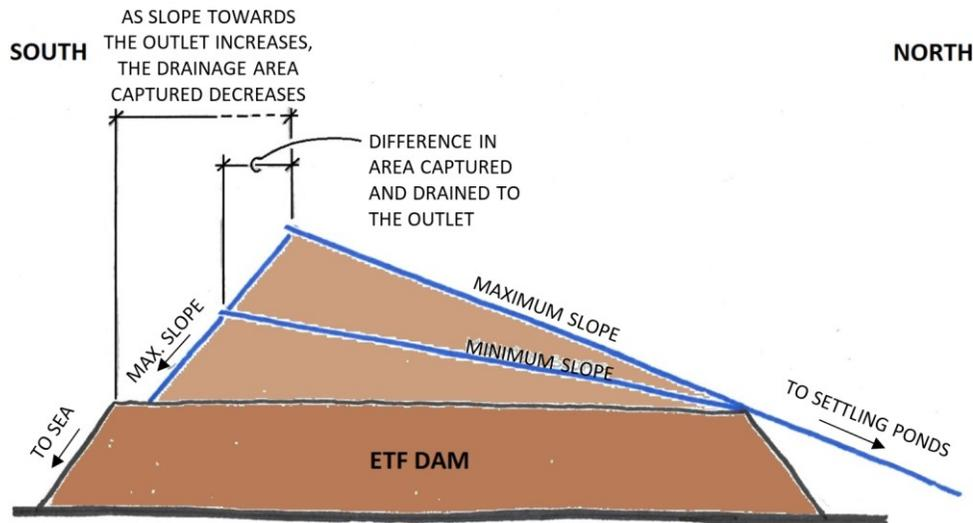
Figure 3.11 Schematic of how slope towards north outlet affects the proportion of water captured and directed to the north outlet. Not to scale.
