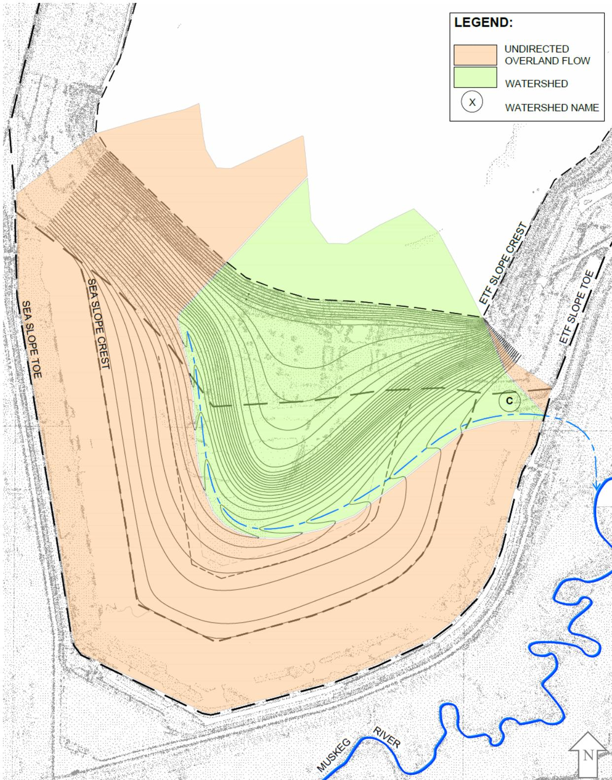
Figure A.6 Drainage Basins designed for the SEA Closure Topographic Design Option 'Three'.
