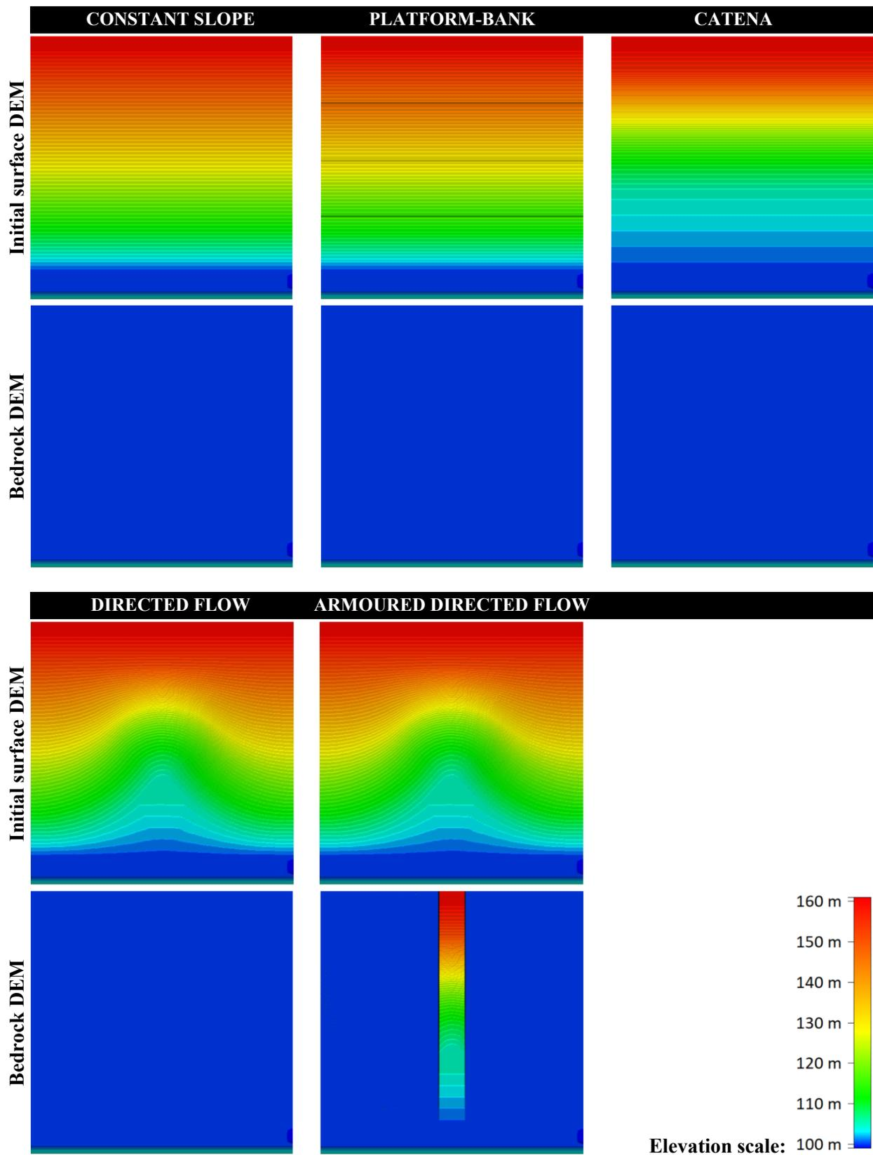
Figure 10.2 Surfacial topography DEMs and bedrock DEMs (500 x 500 m each) for the five dam designs simulated.
