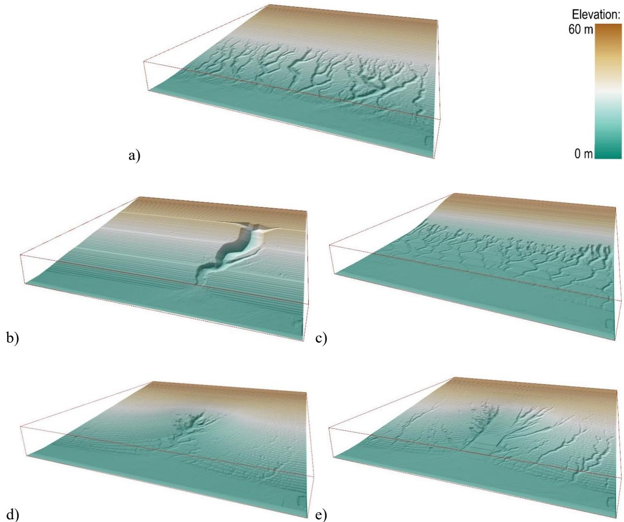
Figure 10.5 Dam designs following stress testing. Shown in three-dimensions (with colour ramp representing elevation): a) constant slope, b) platform-bank, c) catena, d) directed flow, and e) armoured directed flow.
