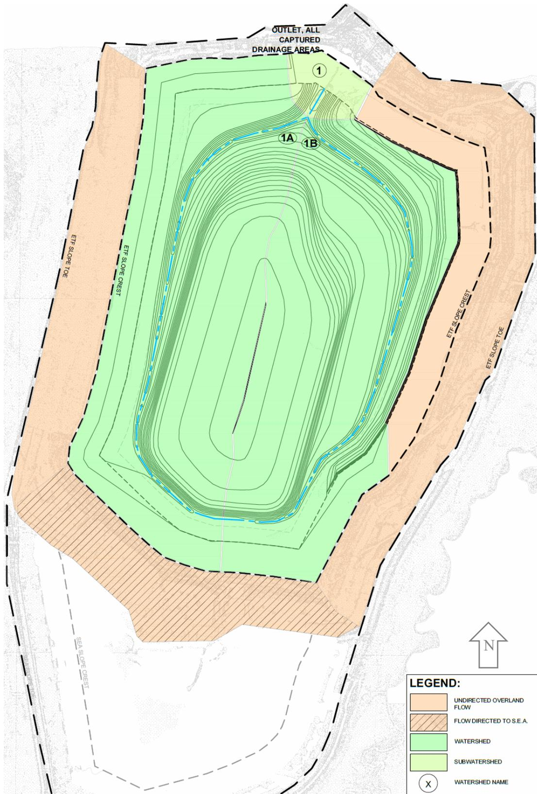
Figure A.3 Drainage Basins designed for the TSF Closure Topographic Design Option 'C' - "Dome".
