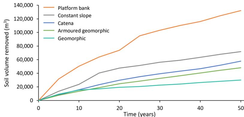
Figure 10.6 Cumulative soil loss from dam designs throughout the stress test
