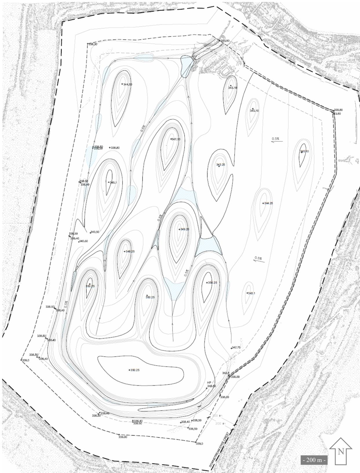
Figure 3.12 Tailings storage facility closure topographic design Option 'A': "drumlins". Volume maximization using 15% maximum slope. Drawing not to scale.
