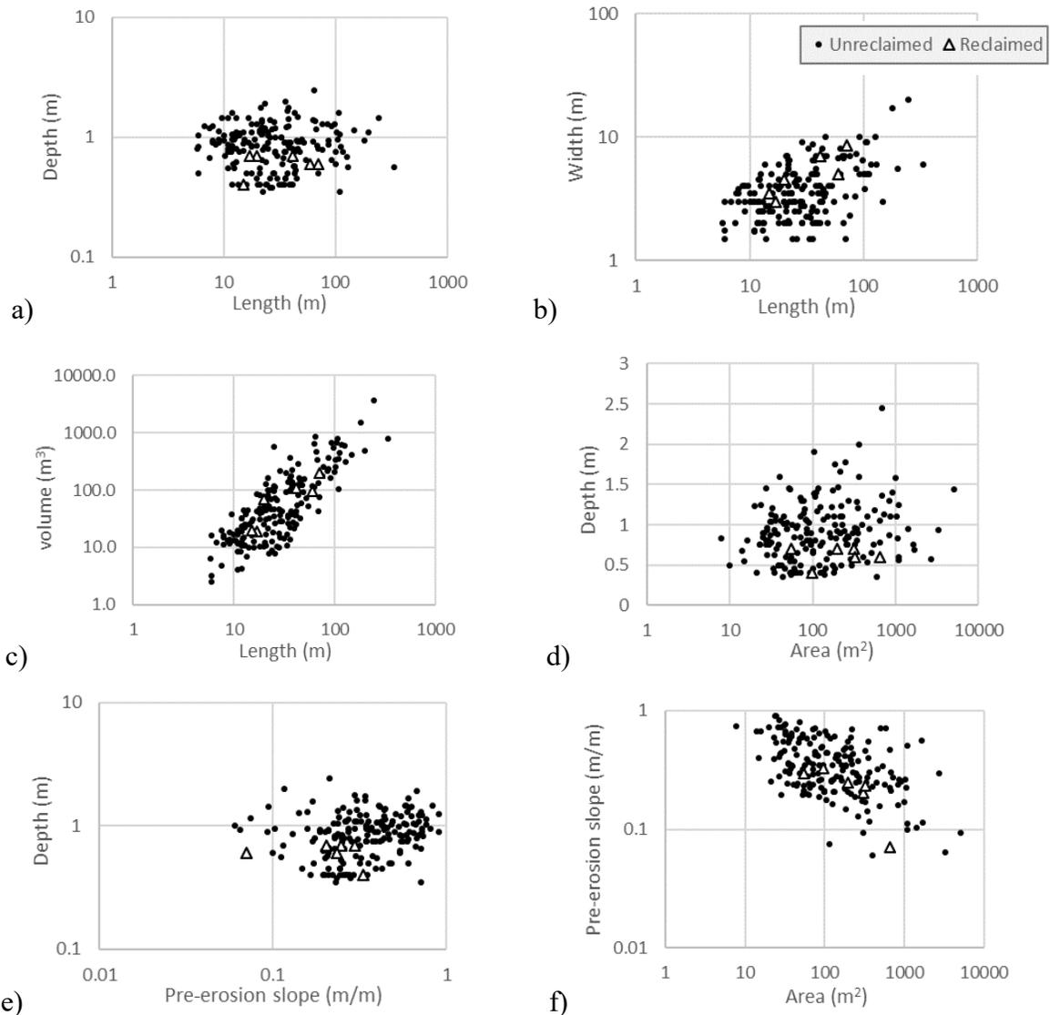
Figure 6.8 Gully length, width, depth, area, and pre-erosion slope characteristics for those found on reclaimed and un-reclaimed dam slopes Slight correlation between volume and length was found, although other properties demonstrated little correlation, perhaps due to the variation in cause.
