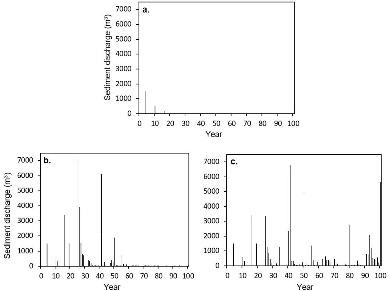
Figure 9.10 Sediment discharge throughout 100-year model: (a) Simulation 'A', (b) Simulation 'B', and (c) Simulation 'C'.
