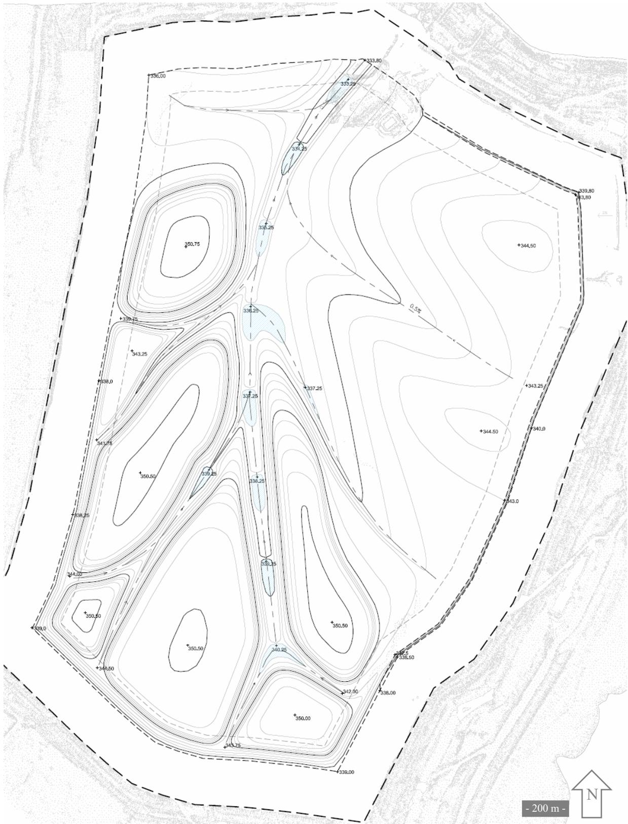
Figure 3.13 Tailings storage facility closure topographic design Option 'B': hummocky ridge and swale". Volume maximization using 15% maximum slope. D
