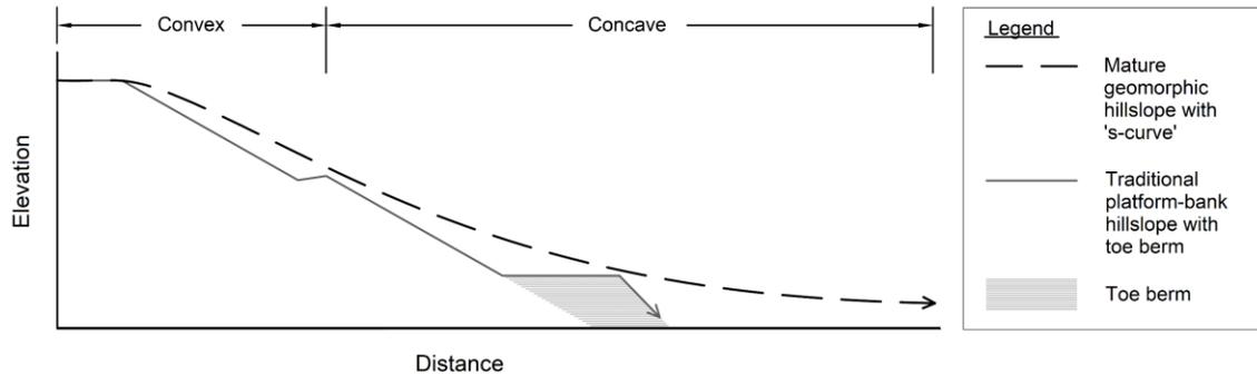
*Figure 4.5 Traditional platform-bank and geomorphic S-curve post-mining slopes. In the platform-bank approach uniform slopes are broken up with oppositely sloped banks, or “benches”. Uniform slopes naturally evolve into concave slopes over long time periods, suggesting this form is more sustainable post-closure than platform-bank geometry. Not to scale. Dimensions and slopes will vary.*
