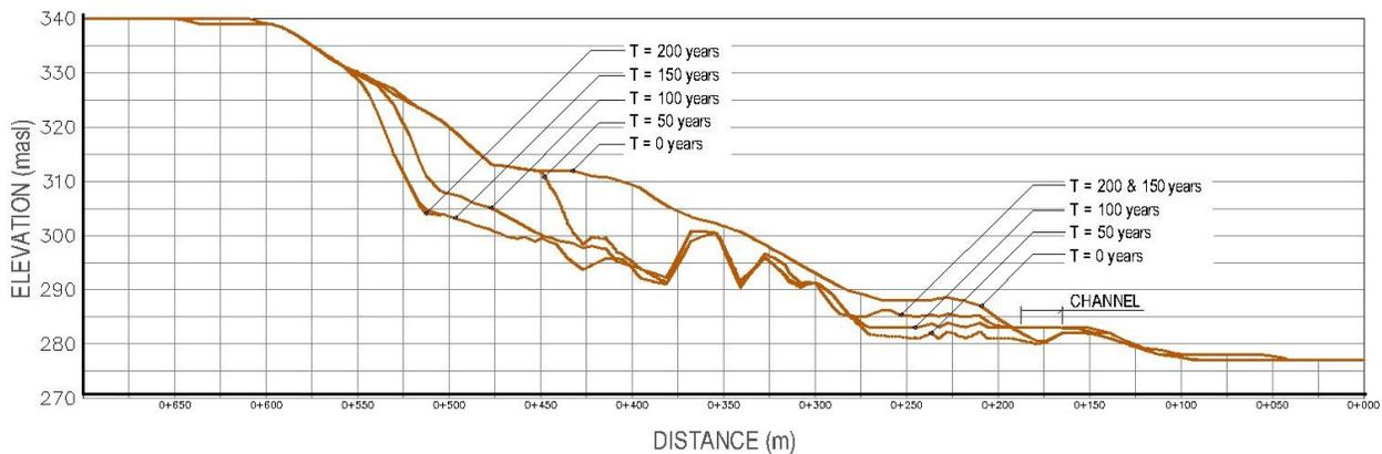
Figure 8.12 Surface profile of an eastern (downstream) portion of a sand dyke prior to landscape evolution modelling (time = 0 years), and after 50, 100, 150, and 200 years of simulation. 3x Vertical exaggeration, profile is not to scale.
