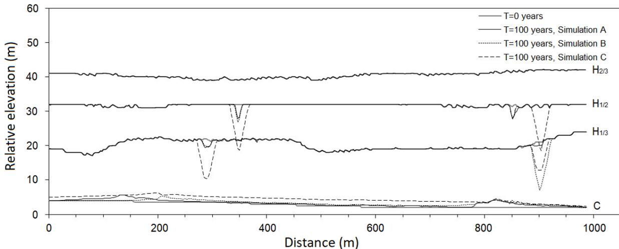
Figure 9.8 Sections through the downstream face of a roughly 1 km section of the dam prior to simulation ( $T=0$ , solid line), and following 100 years of Simulation ‘A’, ‘B’, and ‘C’. Sections taken at the toe (in channel, C), at 1/3 height, 1/2 height, and 2/3 height.
