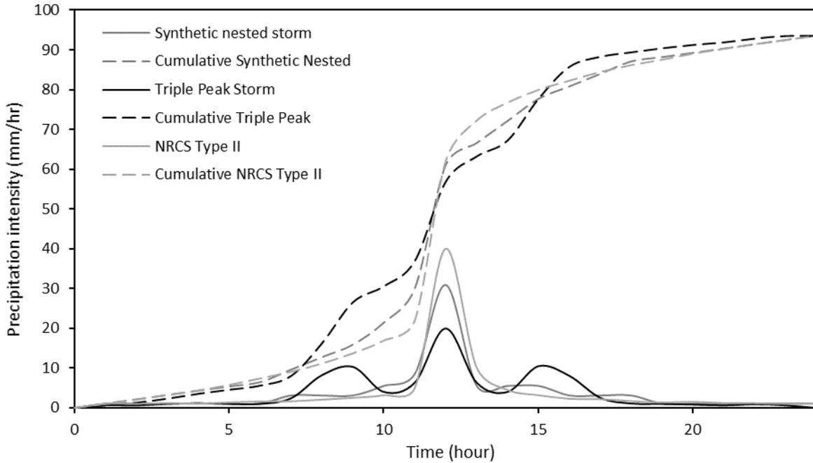
Figure 8.5 Example hyetographs for the historic 1:100 year, 24-hour storm in Ft. McMurray using the NRCS Type II distribution typically used in the region, the synthetic nested storm distribution used in areas where no distribution is specified, and the triple-peak distribution fitted to Ft. McMurray by (Dick & Ghavasieh, 2015).
