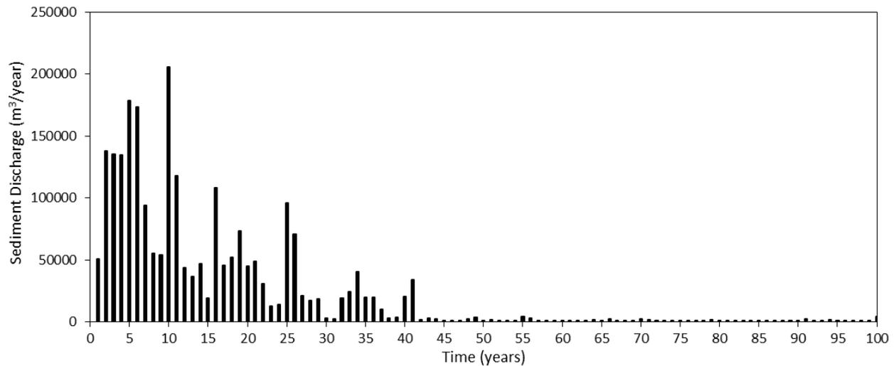
Figure 8.11 Annual sediment discharge from entire TSF over the first 100 years of simulated landscape evolution. Note: 50,000 m<sup>3</sup> of CST is approximately equal to 80,000 tonnes.
