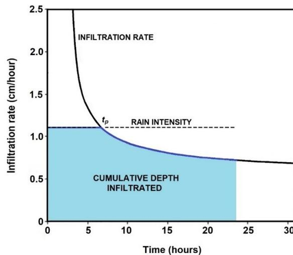
Figure 5.2 Infiltration rate changes over time, as shown using the Green-Ampt equation (5.4) above.
