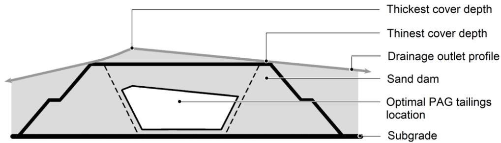
Figure 4.7 Distance from outlet and corresponding cover thickness. Cover increases in thickness with increasing distance from outlet. Potentially acid generating (PAG) tailings are placed here according to cover thickness.
