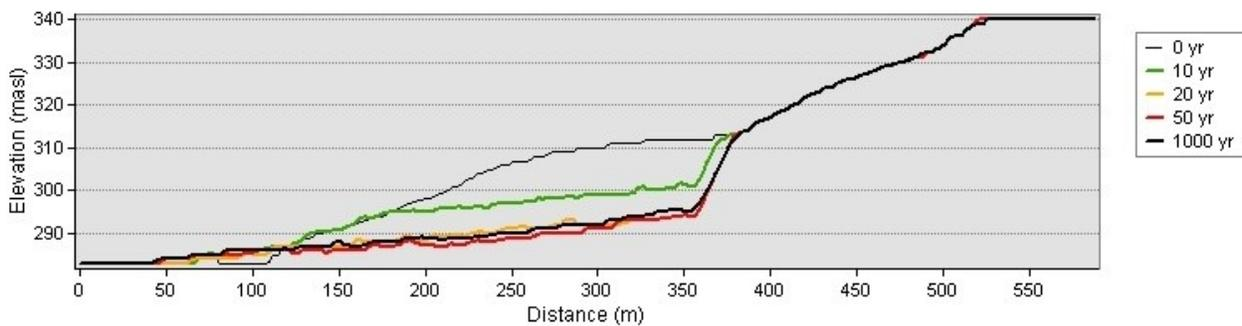
Figure 8.8 Model results: section through a gully formed on an AOS sand dam with toe berm over 1000 years
