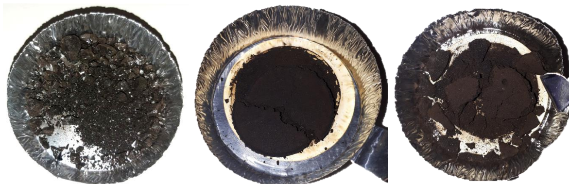
Figure 3-1: Appearance of Raw Asphaltene, n C5 and n C7 40:1 Insoluble (from left to right)
