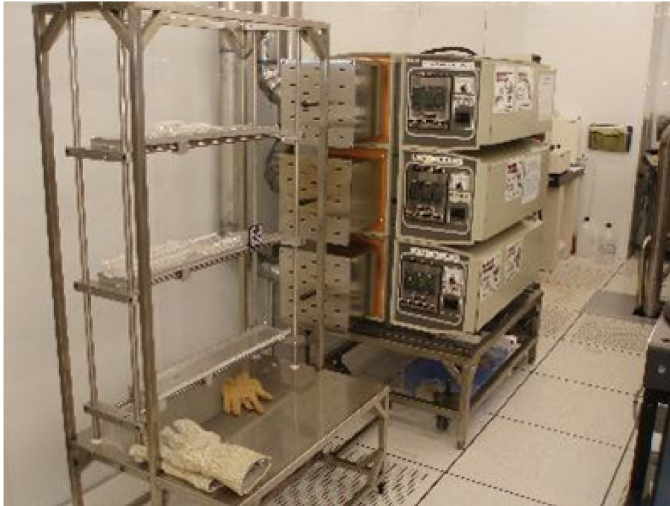
Figure 4-6 Thermal wet oxidation furnace
