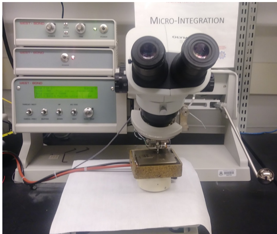
Figure 5-8 A wire-bonder, West.Bond® 7476E
