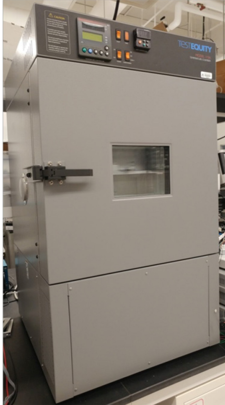
Figure 5-3 Thermal load calibration setup including environmental chamber, source meter, and switch box
