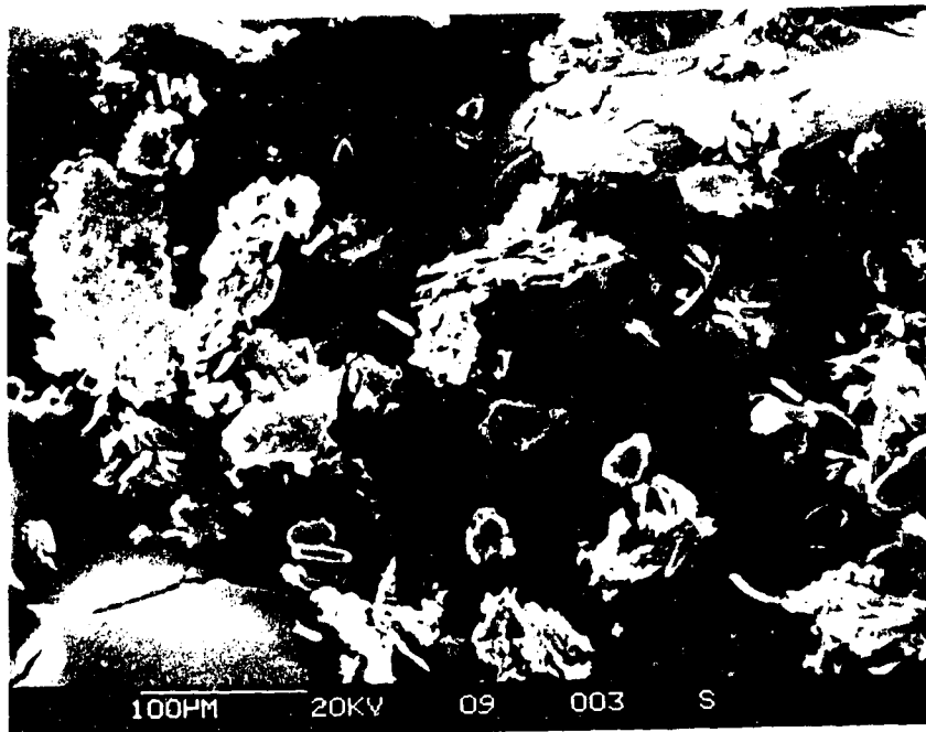
Figure 2.7(iii) SEM Photomicrograph of Granular Cellulose Taken After Sonication in Water for 1 hr.
