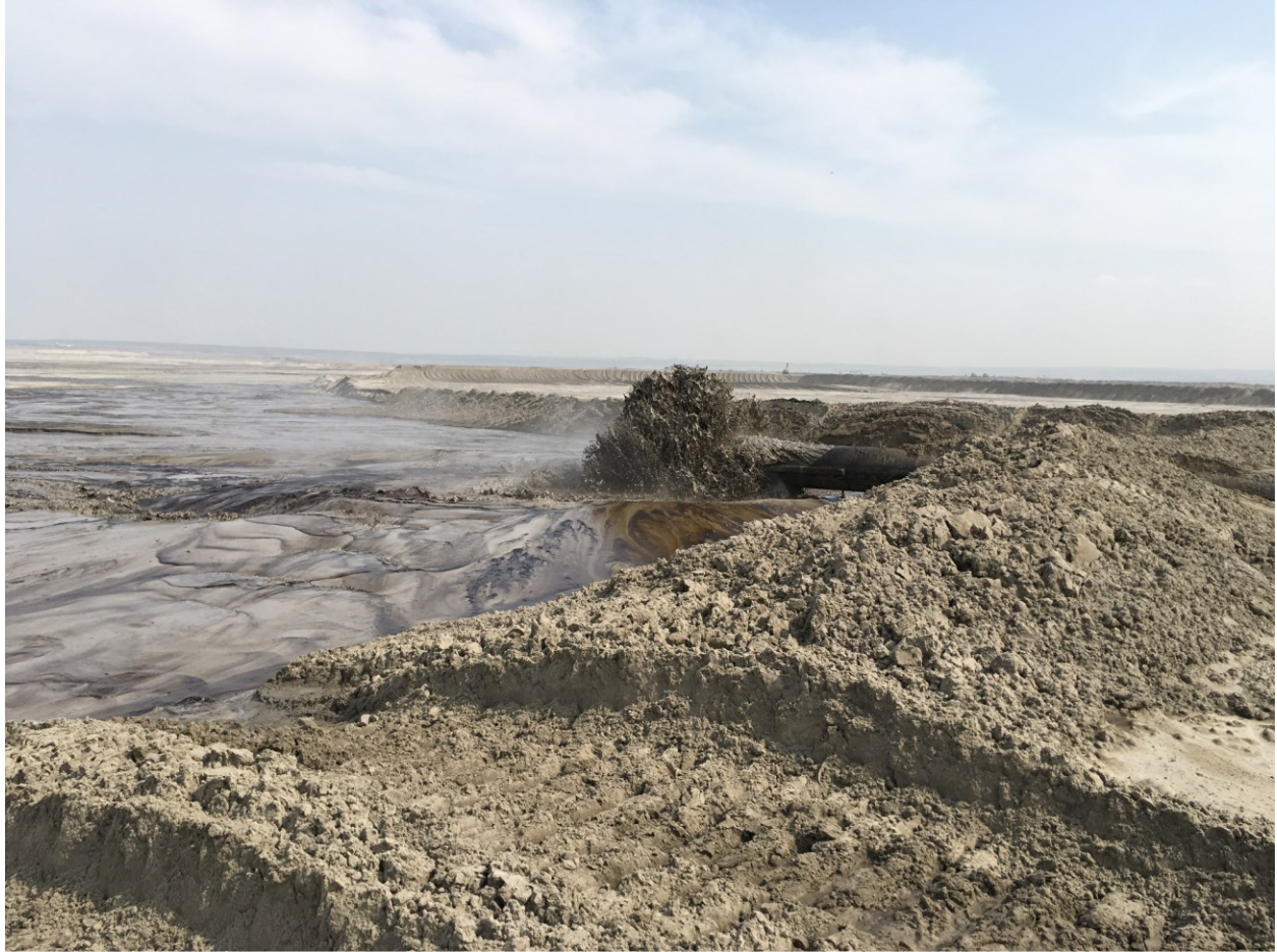
Summer Photo (c), Table 7. View of tailings discharge area and end of line device (dissipates kinetic energy).
