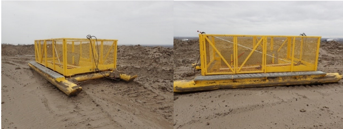
Figure 20. Rescue skids for a tailings discharge area that can be hooked up to a bulldozer.
