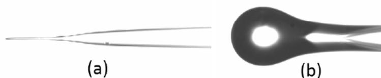
FIGURE 2.2: Substrate preparation images: a) a sharp micro-pipette tip obtained after stretching in hot-wire puller; b) the substrate is further melted until a sphere of desired size is acquired
