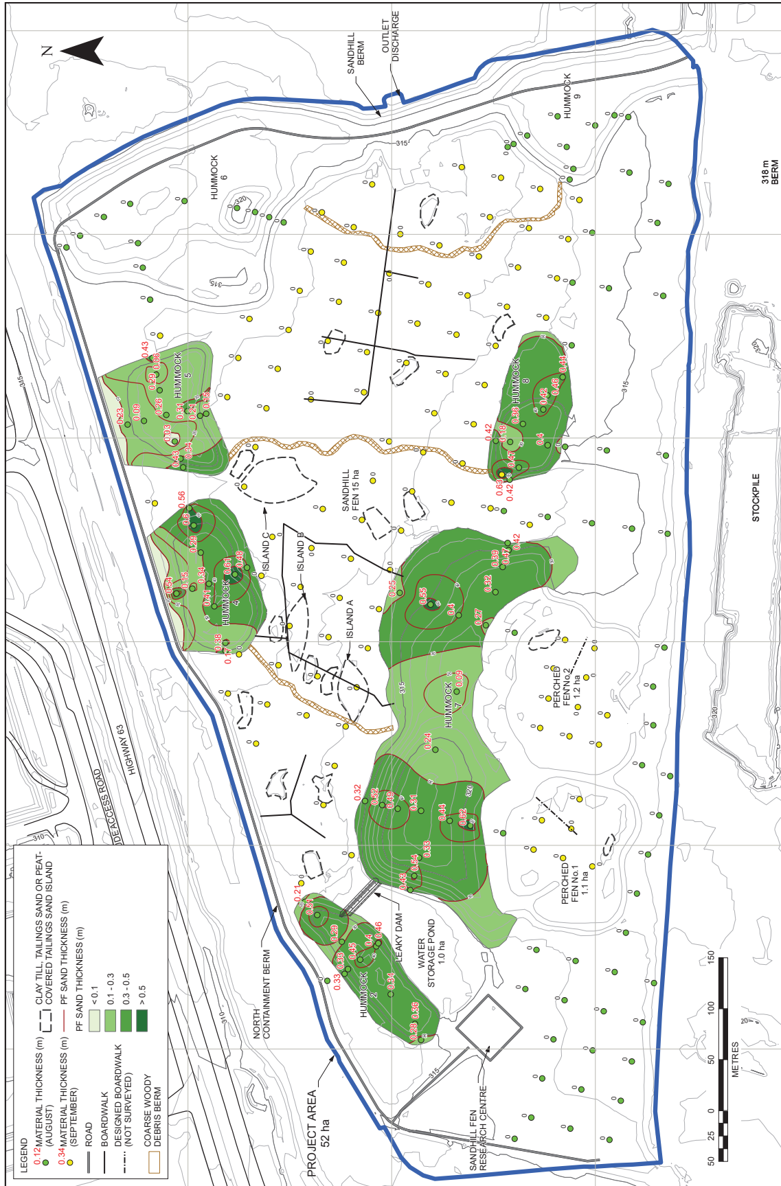
Figure A-7: Isopach map of PF sand subsoil prescribed to hummocks 2, 4, 5, 7, and 8.
