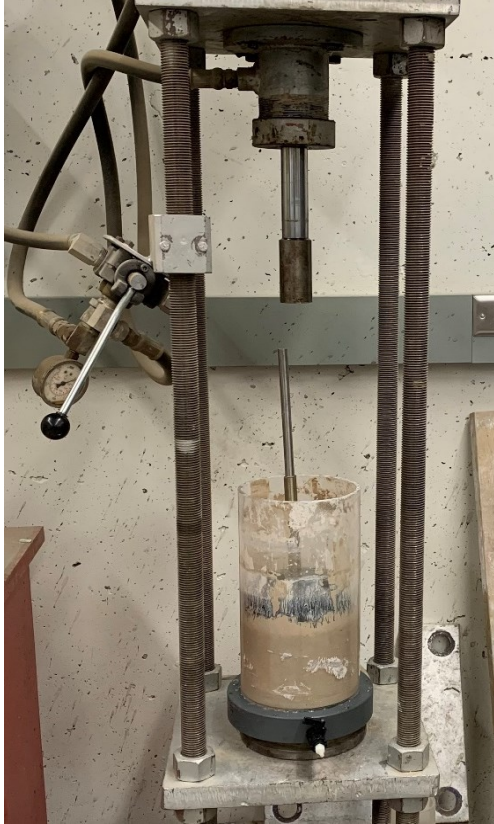
Fig. C4: Procedure used for obtaining cylindrical fiber-reinforced samples from the slurry for triaxial testing
