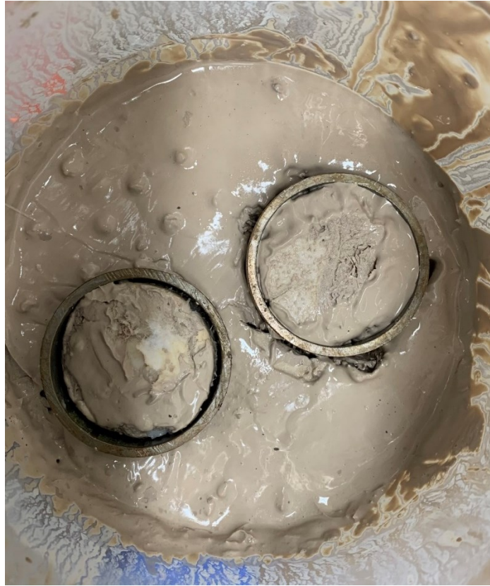
Fig. C4: Procedure used for obtaining cylindrical fiber-reinforced samples from the slurry for triaxial testing
