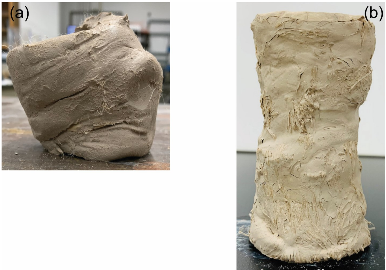
Figure 6.6. Slurry prepared fiber-reinforced samples after failure in (a) compression test and (b) extension test.
