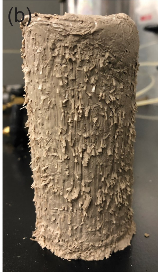
Fig. C5: (a) Slurry prepared unreinforced soil (b) Slurry prepared fiber-reinforced soil
