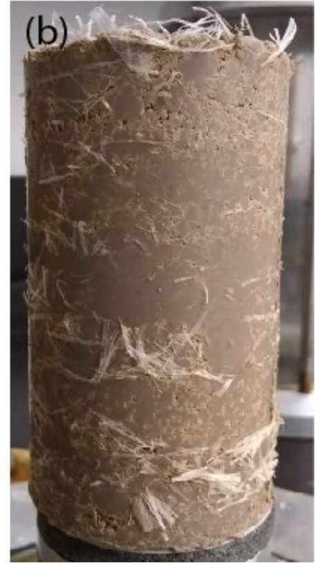
Fig. C2: (a) Prepared fiber-reinforced soil lot (b) Compacted fiber -reinforced sample used for testing
