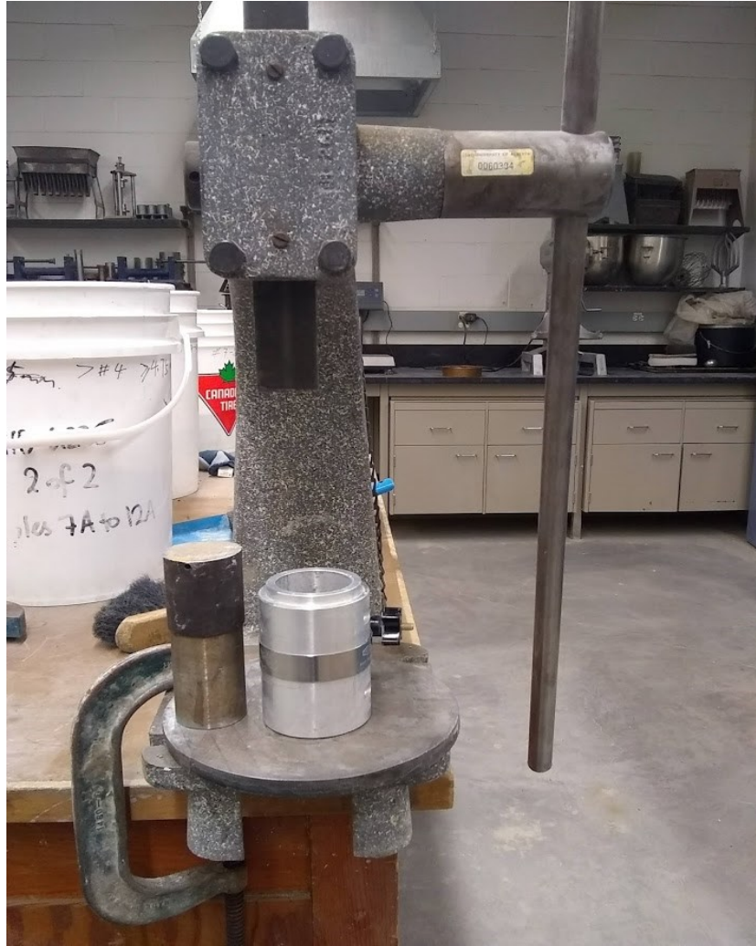
Fig. C1: Apparatus used for preparing compacted fiber- reinforced samples including arbor press, 2-part compaction mold and hammer
