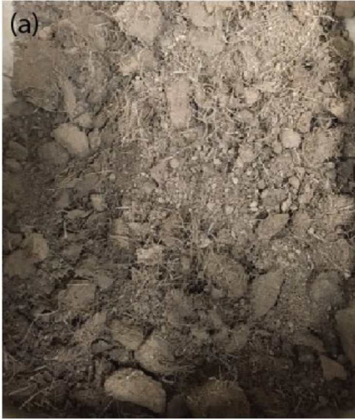
Fig. C2: (a) Prepared fiber-reinforced soil lot (b) Compacted fiber -reinforced sample used for testing
