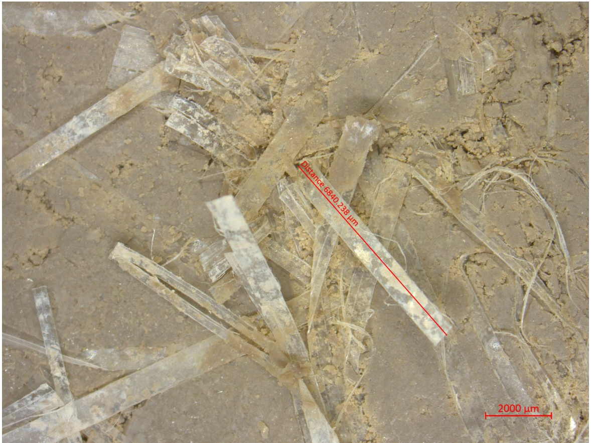
Fig. D1: A section of the prepared fiber-reinforced specimen observed using the optical microscope Zeiss AXIO Lab.A1
