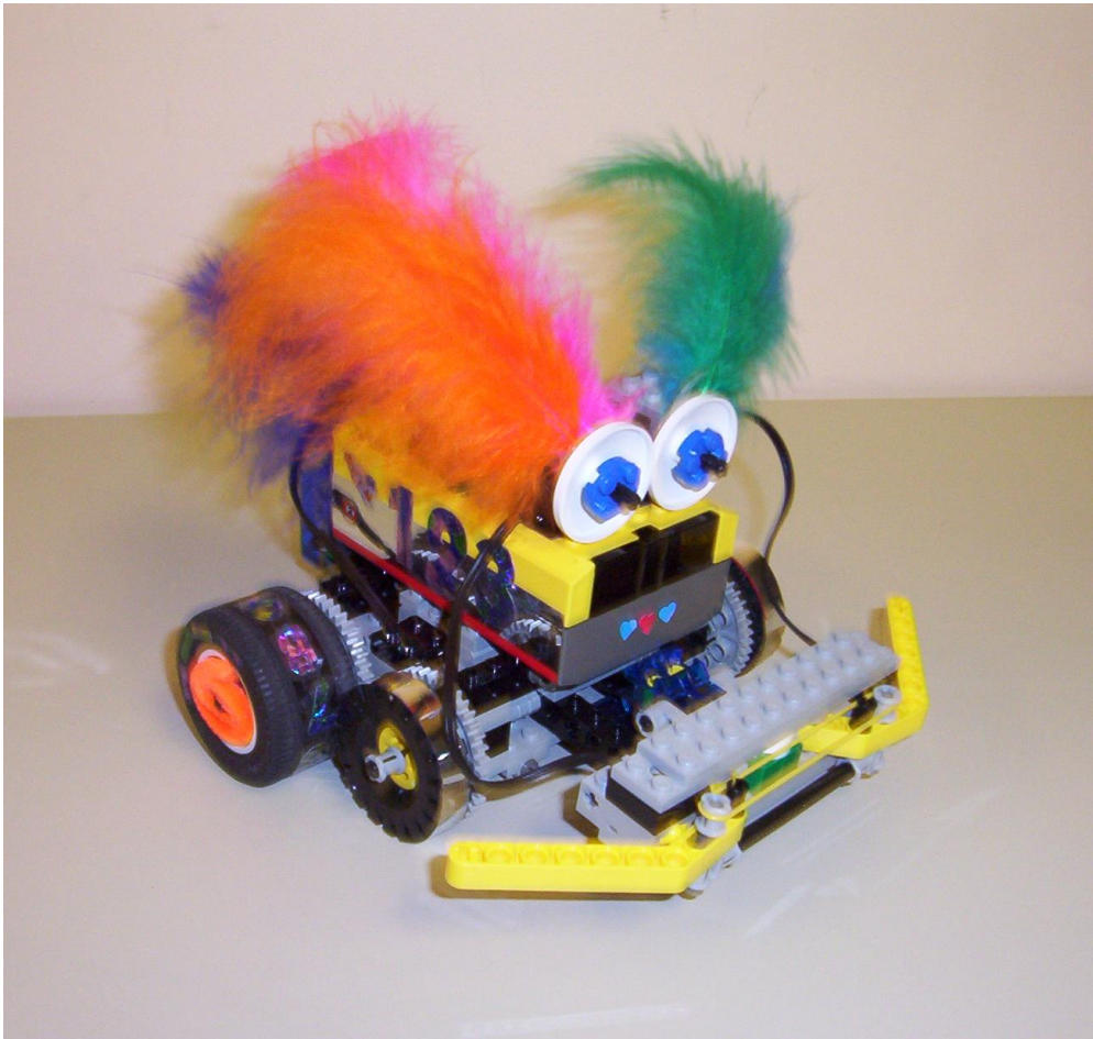
Figure 1. Lego RCX Mindstorms roverbot, a car-like robot
