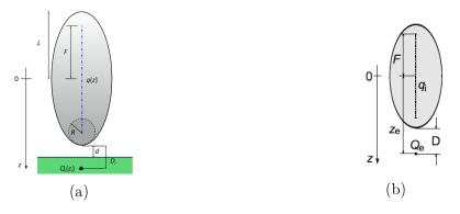
Figure 5.4: (a) Spheroid dipole dimensional parameters. (b) Schematic showing how the field and scattering by a spheroid can be calculated by approximating charges at various points. The tip-sample distance is d, radius of the base of the ellipsoid is R, major axis radius is L and the focal distance is F. Adapted from [127].
