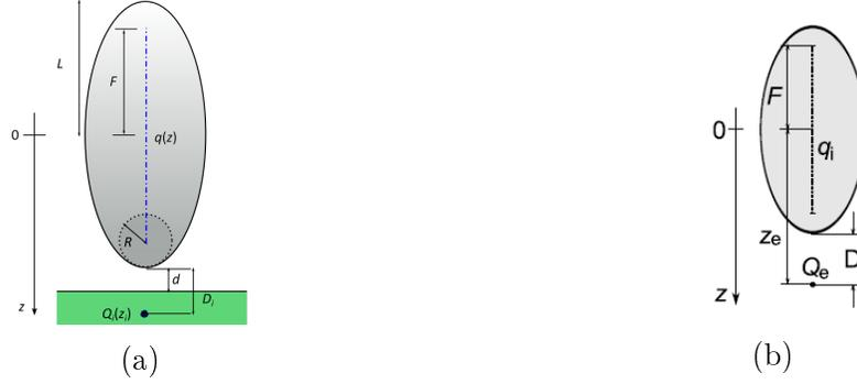
Figure 5.4: (a) Spheroid dipole dimensional parameters. (b) Schematic showing how the field and scattering by a spheroid can be calculated by approximating charges at various points. The tip-sample distance is  $d$ , radius of the base of the ellipsoid is  $R$ , major axis radius is  $L$  and the focal distance is  $F$ . Adapted from [127].
