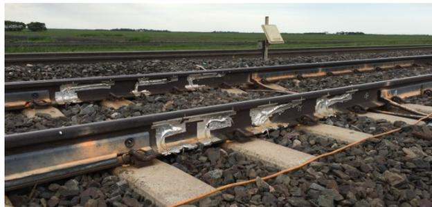
Figure 6-3 A photo of the WILD system and instrumented cribs along the north track at the Calrin site.
