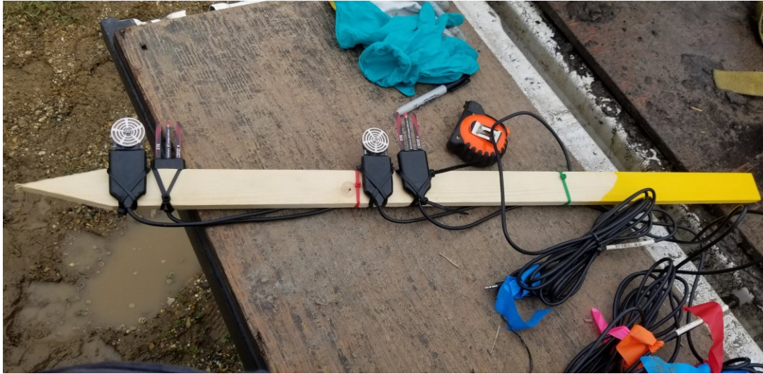
Figure 4-1: Photo showing Decagon 5TE and MPS-6 sensors at 25 and 50 cm depths attached to stake before placement in tailings-filled totes
