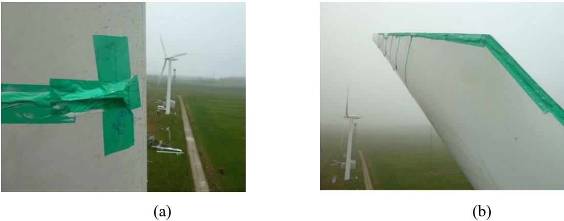
Figure 2-37: Blade monitoring using vibration method with acceleration sensors [139]
