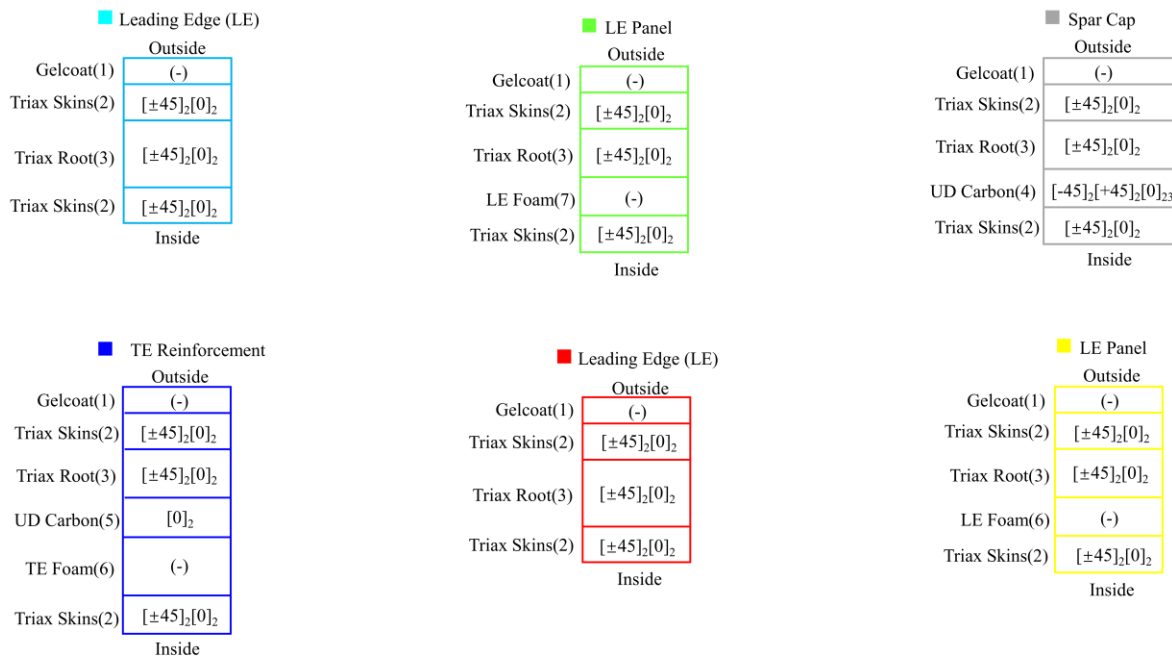
Figure 3-5: Material zone definition for Station # 13 of the 5-MW blade in the chordwise direction
