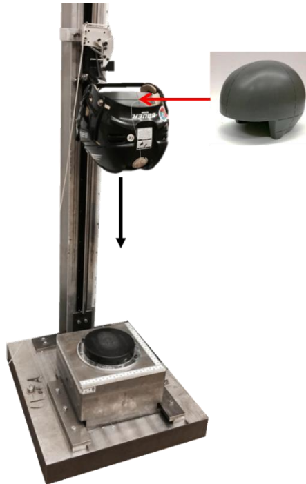
Figure 2.3: An example of a hockey helmet certification set-up with a helmeted magnesium headform (EN960) and rigid neck, striking a modular elastic programmer (MEP) pad. The position shown is prior to release.
