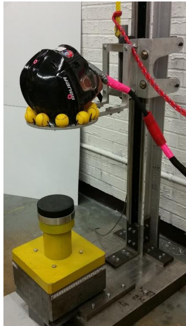
Figure 3.7: The drop tower configured for hockey helmet impacts with Hybrid III head without a neck. A custom gimbal attachment designed for no-neck impacts is used here.
