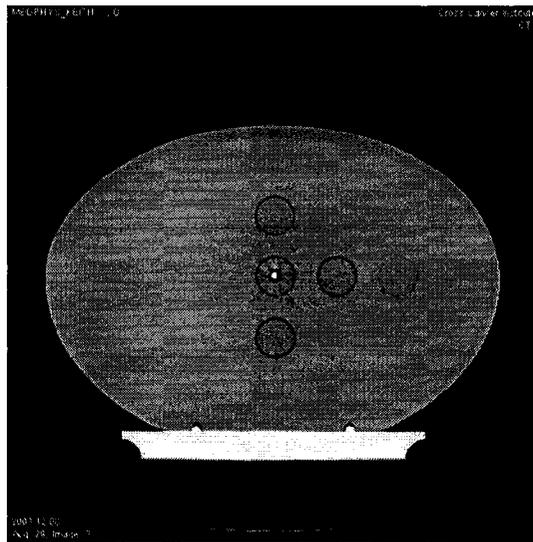
(b) CT image showing the air gaps surrounding the rods and cable in the CIRS phantom leading to a reduction in the SSDP values for  $z > 0$ .
