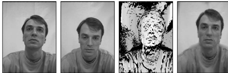
(b) An example of the result. From left to right: bottom view, top view, disparity map, and virtual image
