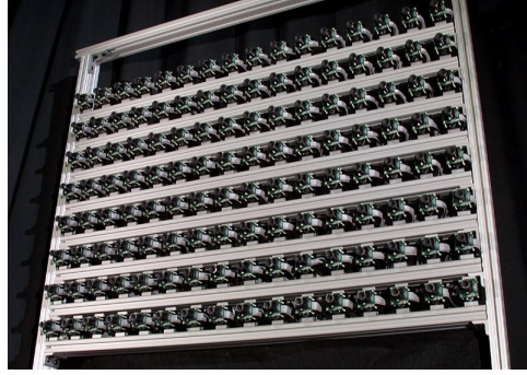
Figure 2.21: Camera array for a Light Field system [83]
