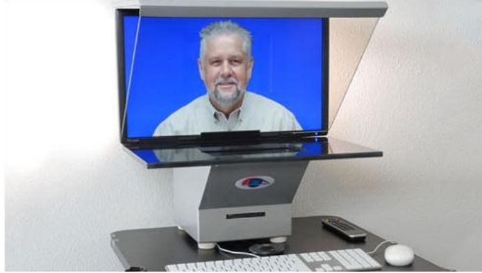
Figure 2.3: A demo of Eye-to-Eye systems: TPT 22 desktop (from: http://www.telepresencetech.com/tpt22-desktop )
