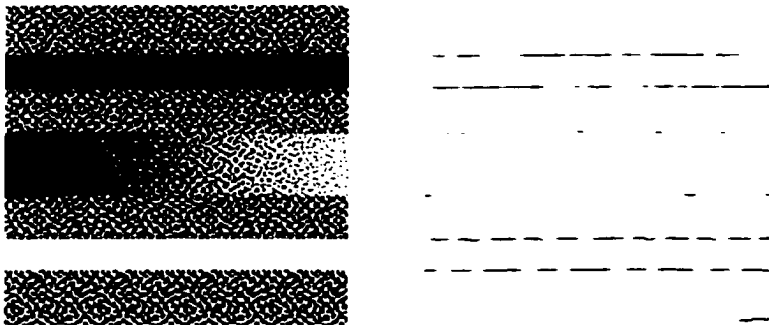
Figure 6.6: Edge distortions produced by clustered dot halftoning algorithms. Halftoned images printed at 150 dpi are presented in the left column. The right column presents an image distortion errors for significant edges at a scale 4
