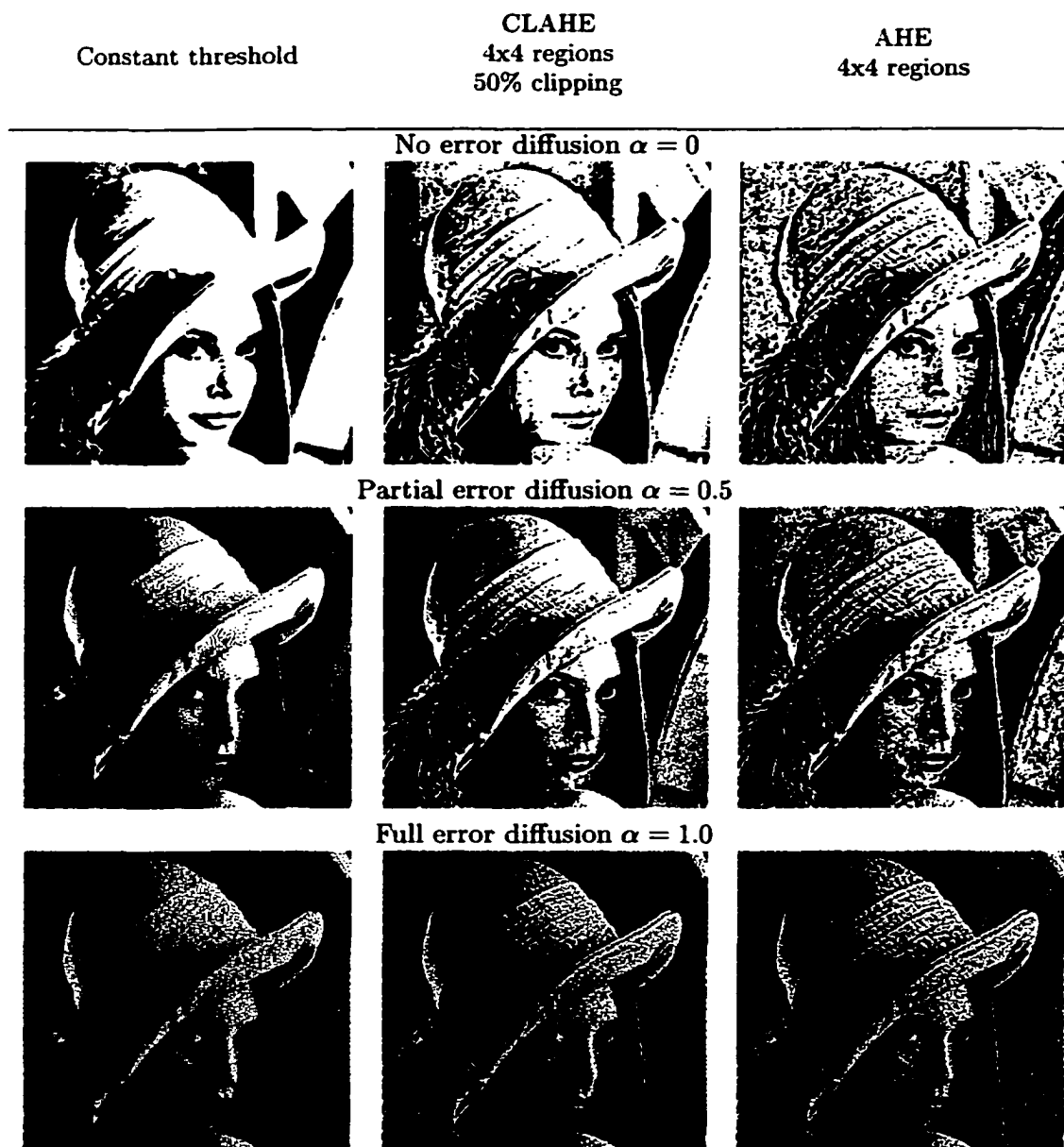
Figure 6.1: The effect of error diffusion depends on the thresholds used for halftoning. The left column corresponds to the constant threshold and demonstrates Floyd-Steinberg [FS76] (bottom image) and Eschbach-Knox [EK91] (center image) approaches. I use dither screens generated by the AHE and CLAHE algorithms to enhance the display of the original image details. However, due to correlation between these screens and the reproduced image, the tone reproduction is inaccurate (top row). The use of error diffusion improves tone reproduction and avoids the distortion of image details. The noise artifacts resulted from the enhancement of textures by the AHE algorithm and are controlled by clipping histogram values in the CLAHE algorithm (center column). These images are printed at 150 dpi.
