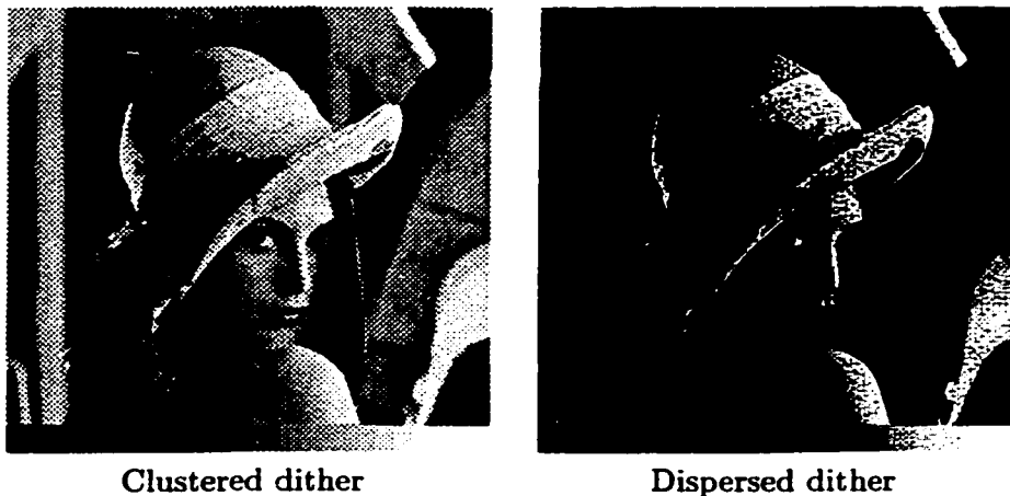
Figure 2.2: Distribution of thresholds in the dither matrix defines the appearance of texture that is introduced into the halftoned layer. Clustered dither produces strong texturing artifacts. Texturing is less visible in the image with dispersed dither. Due to the fact that printers cannot set isolated pixels, clustered dither tone approximation is better than the one produced with dispersed dither matrix. Isolated pixels in the image on the right “bled” into the white space resulting in a strong shift of image contrast.
