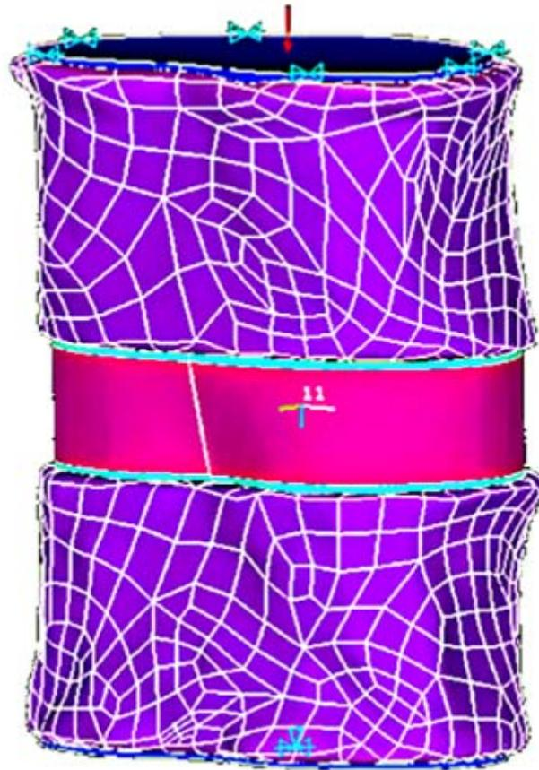
**Figure 5-47: The FSU loading conditions with a pressure load shown in red and the constraints shown in teal**
